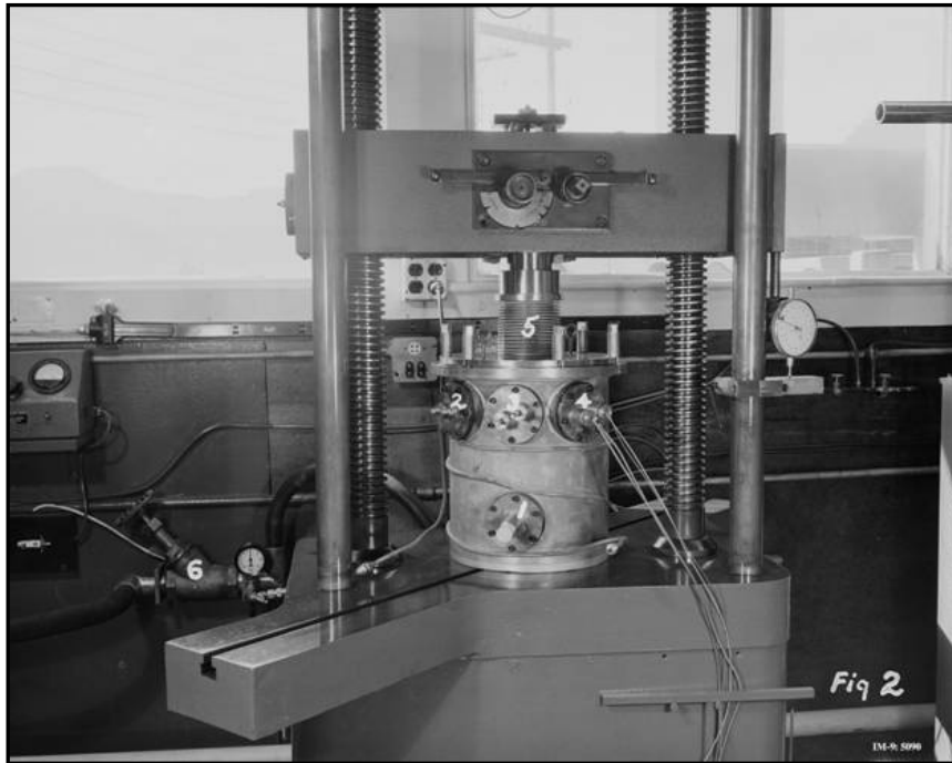
Fig. 4-11. Evacuated hot presses like this were used to form hemispheres of plutonium (Photo IM-9:5090 courtesy of LANL)
