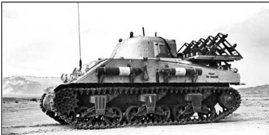
Fig. 10-7. One of two lead-lined tanks prepared to recover soil samples from near ground zero
