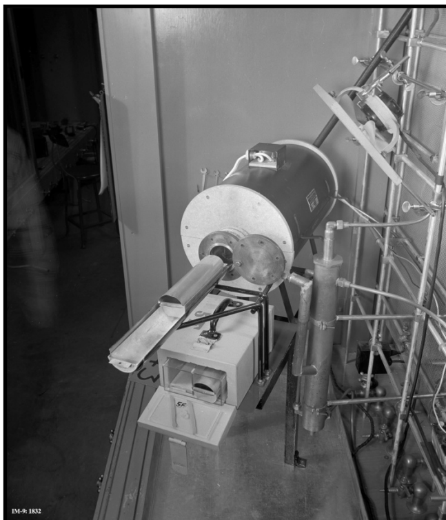
Fig. 4-9. A furnace that was used for fluorination and oxidation reactions (Photo IM-9: 1832 courtesy of LANL)
