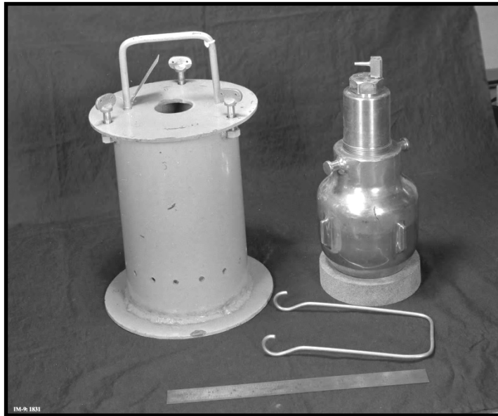
Fig. 4-6. Plutonium was received from Hanford in 80 g and 160 g batches in "shipping bombs" (right) as a slurry of plutonium nitrate. Shipping bombs were transported in protective cases shown on the left. (Photo IM-9:1831 courtesy of LANL)
