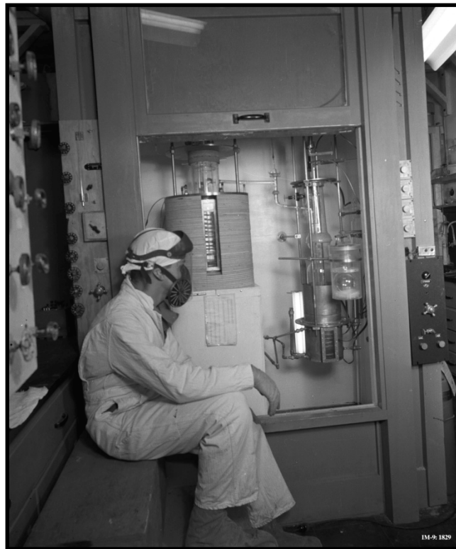
Fig. 4-7. Production-scale purification was conducted in hoods that could be flooded with carbon dioxide in the event of an ether fire. (Photo IM-9: 1829 courtesy of LANL)
