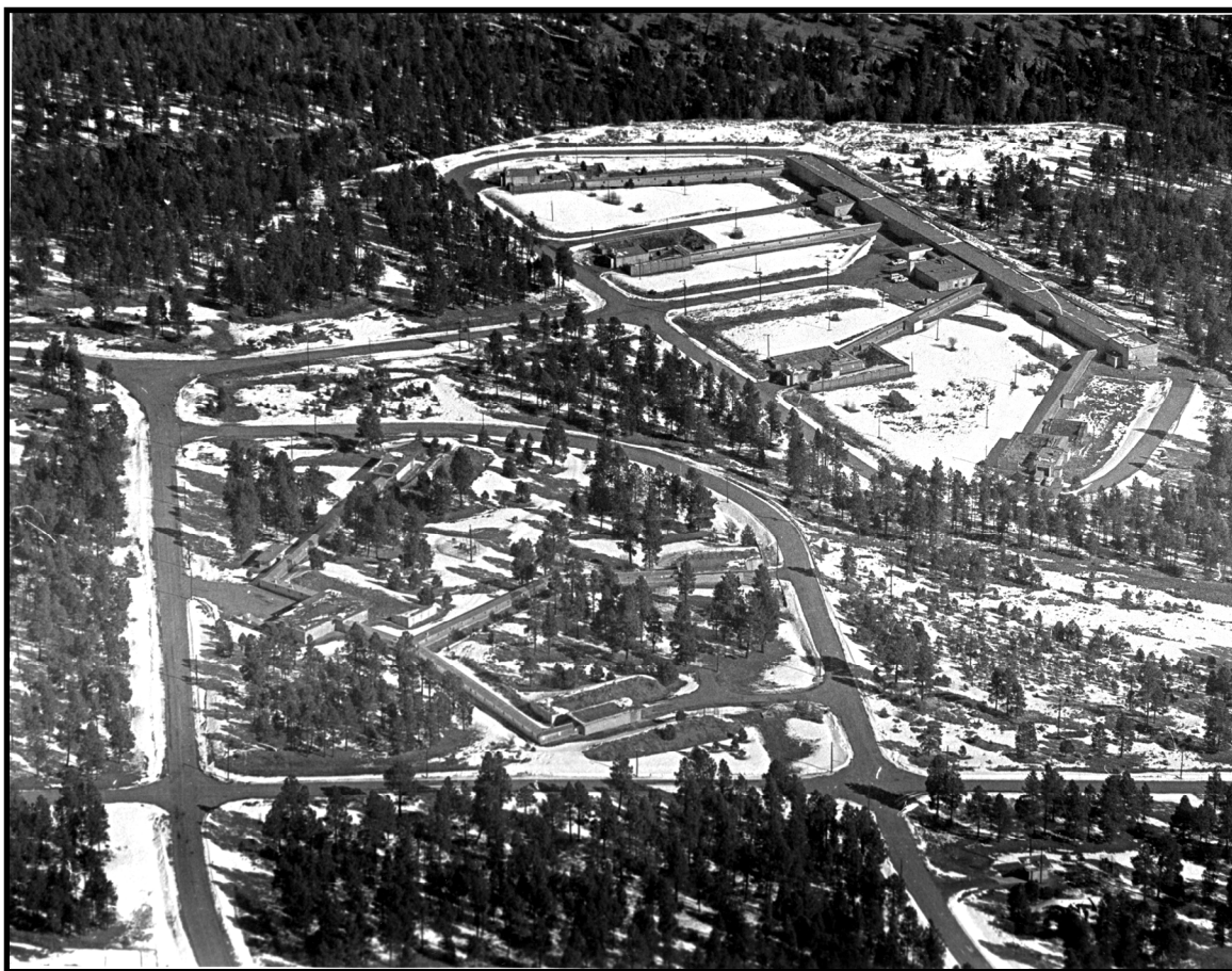
Figure 15-14: High explosives manufacturing facilities were constructed in areas more distant from residential areas than original Technical Area buildings, and wider separation between buildings reflected the more readily recognized safety hazards of associated operations. This August, 1952 aerial view of TA-16 shows Building 260 in the upper right of the image. These buildings for machining high explosives were made of concrete, and had special walls in the back that were built to blow out in the event of an accident. The image shows forested land above and below TA-16. Photo courtesy Los Alamos Historical Society (LAHM-P1990-40-3138).
