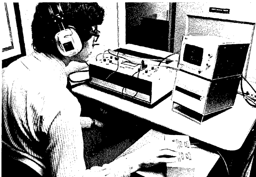
FIGURE 2. Volunteer seated at audiovisual test described in text. The tape recorder is sending auditory signals to the earphones and visual signals to the two channel oscilloscope. Changes in either modality are noted by the subject depressing the appropriate button on the response panel.
