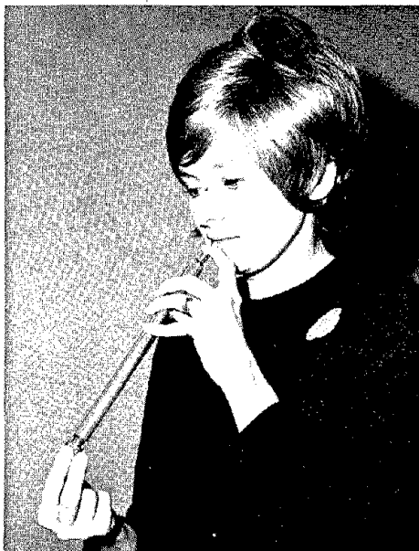
FIGURE 10. The distal cap is secured while the subject is still expiring through the pipette chamber. After the distal cap is secured, the proximal end of the pipette is removed from the mouth and quickly sealed with the finger tip.
