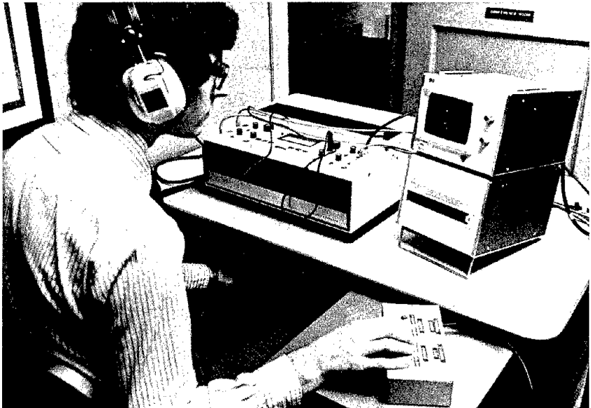
FIGURE 1. Volunteer seated at audiovisual test. The tape recorder is sending auditory signals to the earphones and visual signals to the two channel oscilloscope. Changes in either modality are noted by the subject depressing the appropriate button on the response panel.
