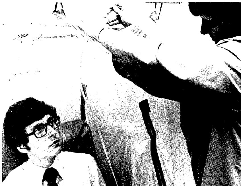
FIGURE 1. Volunteer in exposure tent described in text, through which 70 lpm air is flowing via tubing from above. Ambient air is being sampled from Teflon catheter suspended near subject's breathing zone.
