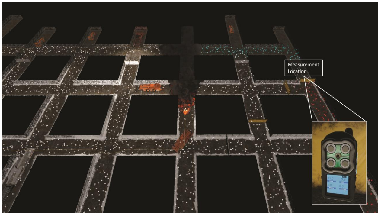
Figure 13. An overhead depiction of a section of a mine with methane liberation coming from the face of the third entry from the right and a fire two crosscuts outby as modeled by MFIRE. The small particle system represents the airflow velocity and methane concentration (i.e., blue = inert, red = explosive, white = none). The dots within the mine indicate level of contaminant by size and color (i.e., larger = higher concentration; red = high, white = none), which would typically be hidden from the user. The callout depicts a multigas detector that users would be able to control to monitor the changes in methane from the location of the star in the overhead view.
