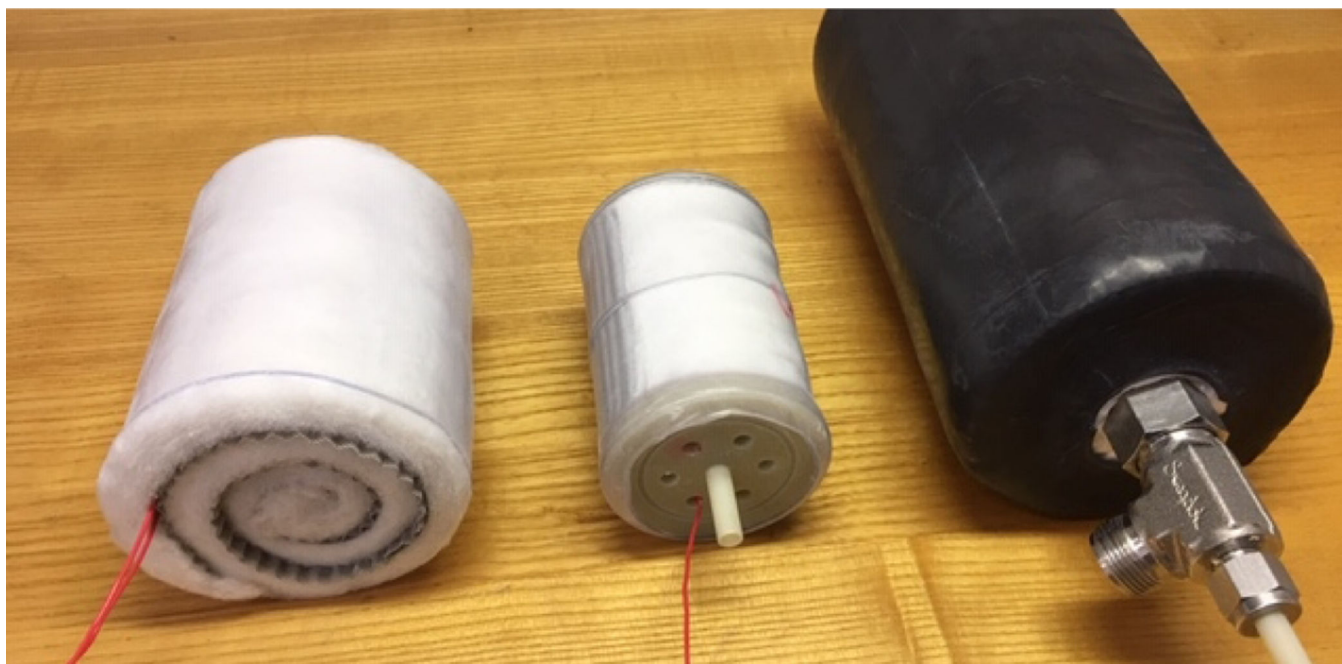
Figure 4. Prototype CFC core modules for cryogenic testing: Module I, Module II, and Module III (from left to right)
