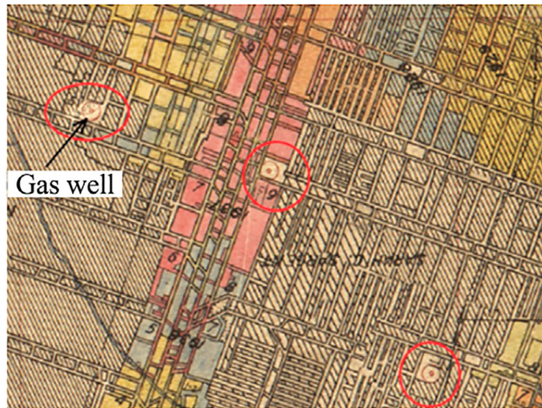
Fig. 1. Portion of a mine map from southwestern PA during the hand-loading era, showing three gas well pillars completely surrounded by pillar recovery.
