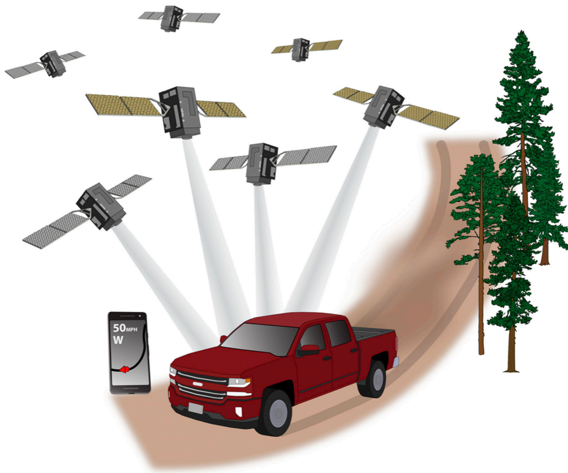
Figure 1. The Global Positioning System (GPS) and, more broadly, the Global Navigation Satellite System (GNSS), rely on three or more navigation satellites to determine ground position of receivers. Position is determined based on the time-delay associated with signal reception relative to synchronized clocks on each satellite. GNSS devices with the capacity to integrate signals from two or more international constellations are increasingly available. The rapidly growing number of satellites generally corresponds with increasing accuracy in a wider range of devices over a 5–10 year transition period.
