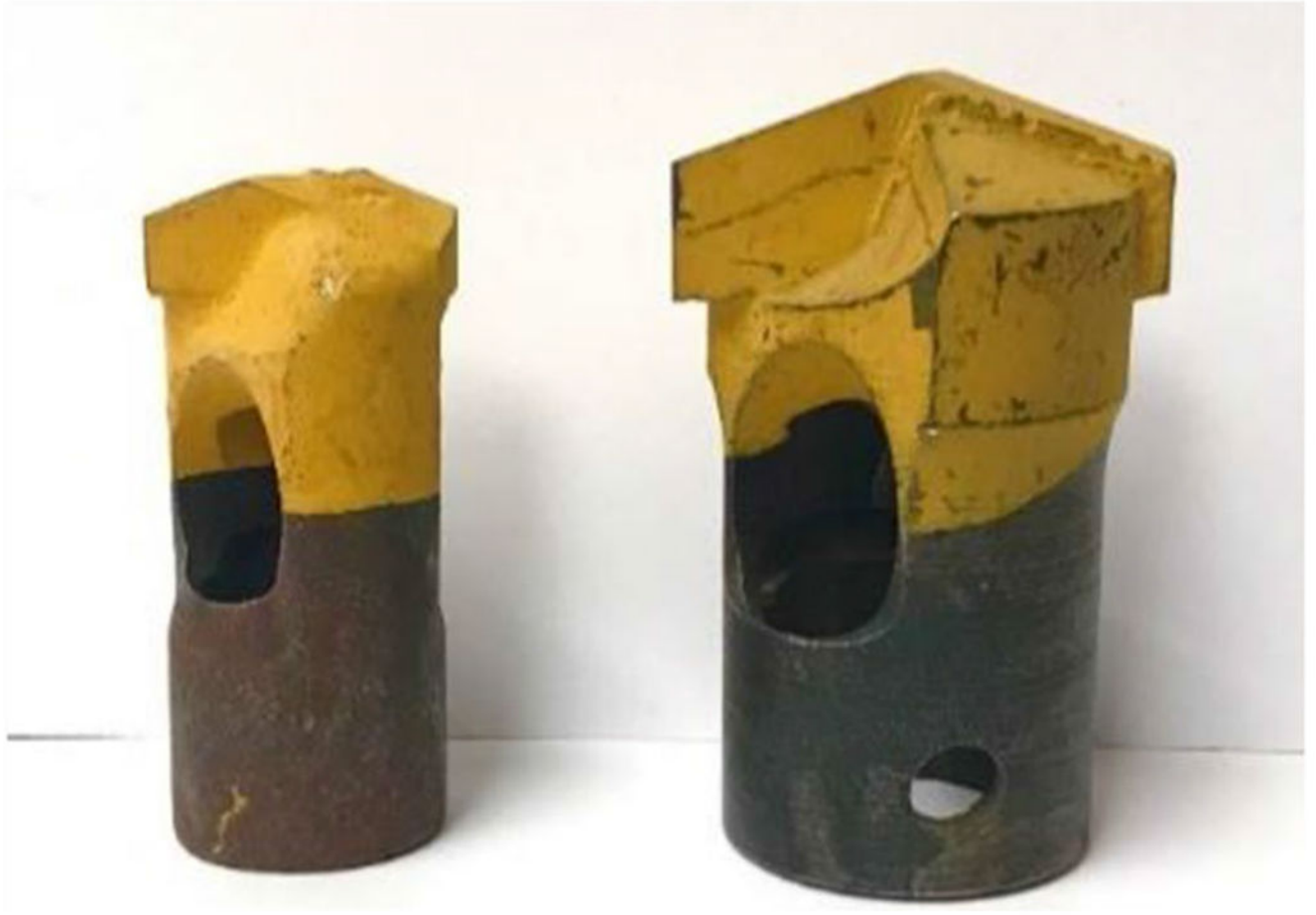
Fig. 2. The tungsten carbide spade bits with 1" (left) and 1-3/8" (right) diameter used
