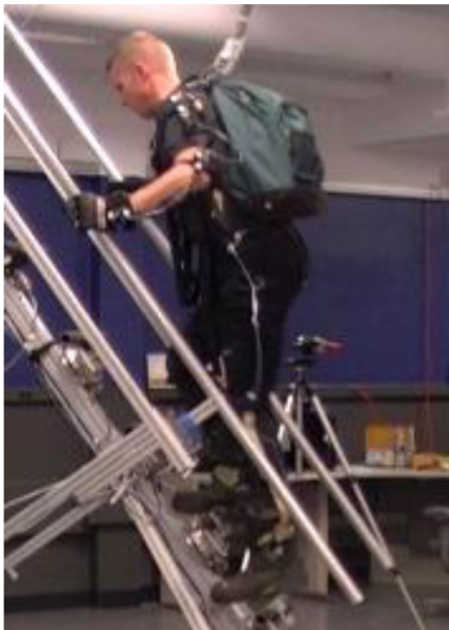
Figure 2: Participant #3 (male, 184.5 cm, 83.9 Kg) climbing a ladder with 356 mm rung spacing at 52.5° angle using “low” 305 mm rails.
