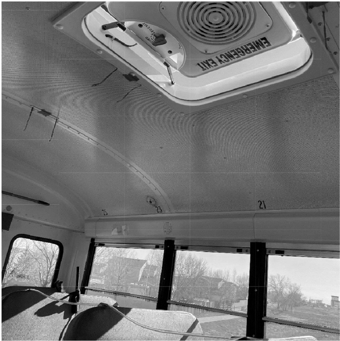
Figure 1. Photo of ceiling hatch fully opened, with the hatch fan on. Passenger windows are closed. A CO 2 probe attached to the back of the bench seat can be seen in the rear of the bus.
