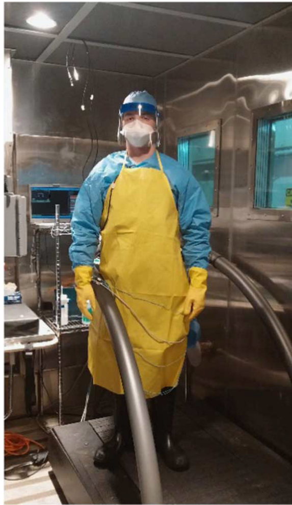
FIGURE 1. Subject Outfitted to Start a Test Wearing the E1 Personal Protective Equipment Ensemble.
