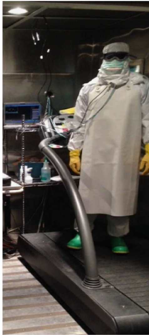
FIGURE 2. Subject Outfitted to Start a Test Wearing the E2 Personal Protective Equipment Ensemble.
