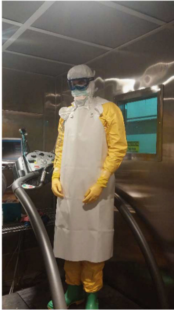
FIGURE 3. Subject Outfitted to Start a Test Wearing the E3 Personal Protective Equipment Ensemble.
