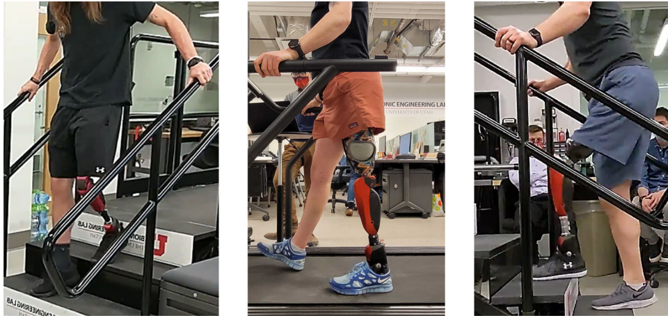
Figure 5. Above-knee amputee participants ambulating with the Utah Bionic Leg. Representative images of the three participants ambulating on the treadmill and staircase.
