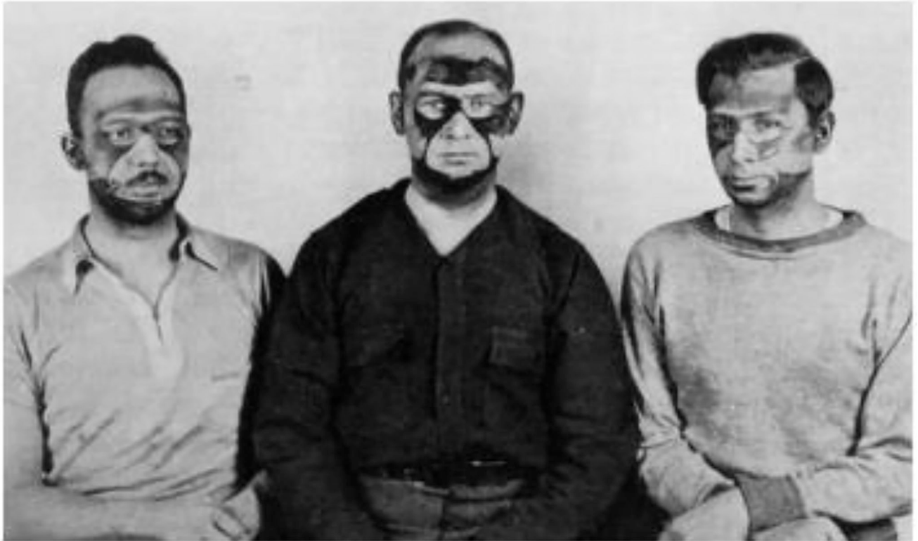
Figure 1. An example of the results of the Direct Leakage and Man Test (the coal dust tightness test) (USDOI 1934).
