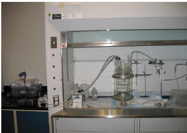
Chamber evaluating direct reading instruments
