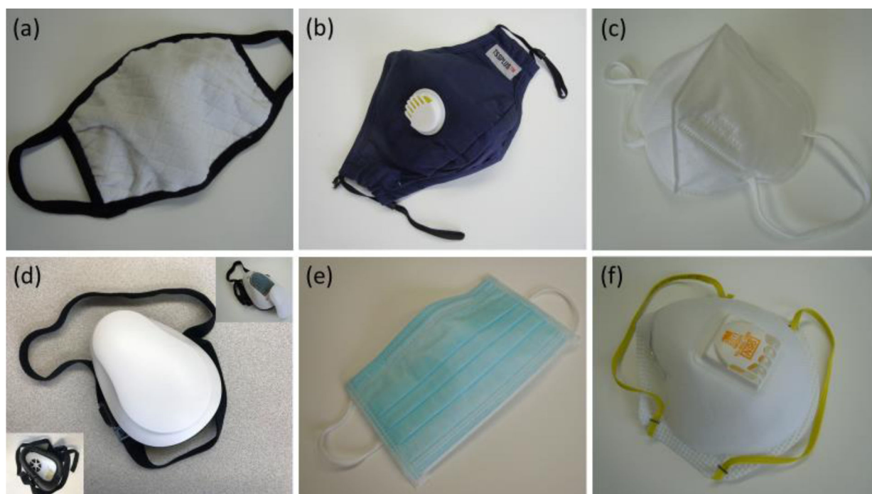
Fig. 1. The loose-fitting masks tested in this study: (a) cloth mask, (b) breathing valve mask, (c) KN95 mask, (d) smart mask, and the two reference masks: (e) surgical mask, (f) N95 mask.
