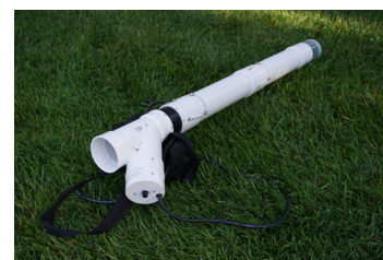
Large, handheld mechanical aspirator removes mosquitoes from natural resting harborage or artificial resting structures.
