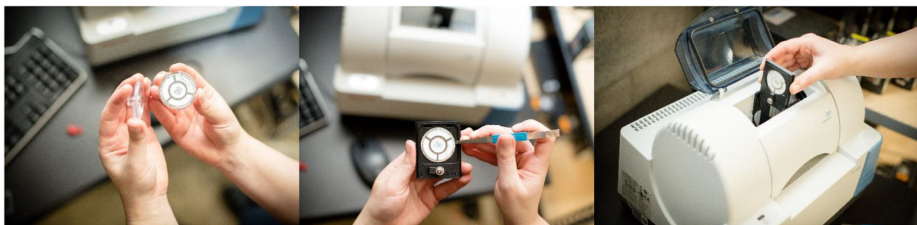
a Opening the cassette b Placing the filter into the filter holder c Loading the filter into the FTIR
