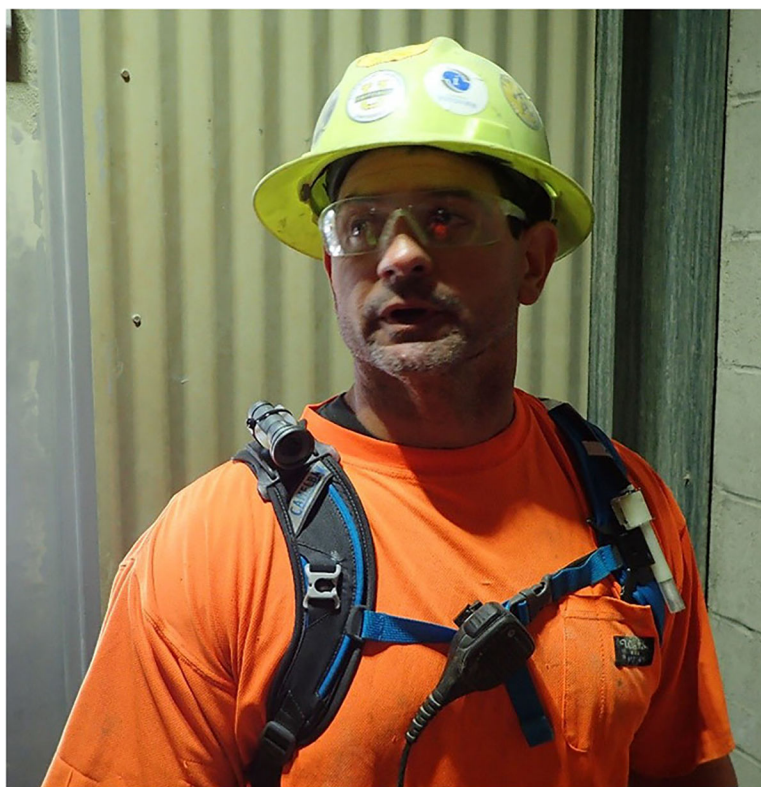
Fig. 1. Photo of video exposure monitoring equipment worn by a miner with mobile camera (right shoulder) and cyclone inlet (left lapel)
