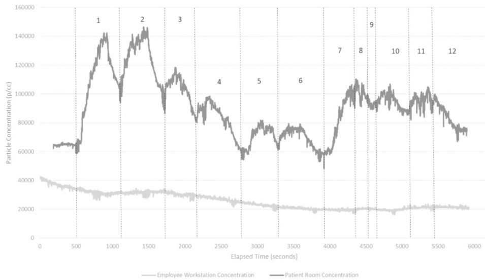
Figure 3. Particle concentration comparison between the PTR and the EWS, from CPC data. The upper curve depicts Particle concentrations in the PTR, while the lower curve depicts particle concentrations at the EWS.
