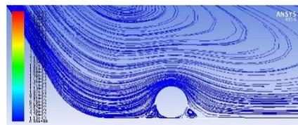
872 **Figure S9** Streamlines for the flow around the cylinder positioned at different locations,  $\theta$ , on
