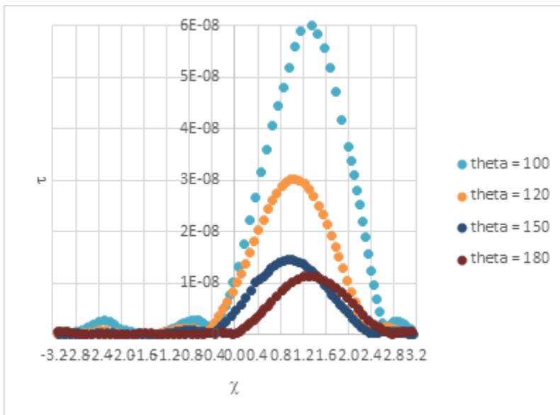
949 **Figure S19** Shear stress  $\tau(\chi)$  around the cylinder, located on the downhill side of the wedge;
