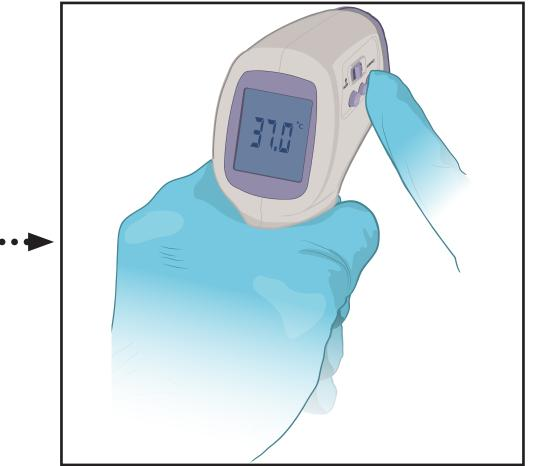
3. Press the button to put the thermometer in Celsius mode. Note: Confirm the thermometer is on "body reading" setting (if applicable).
