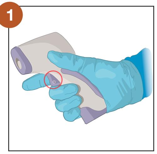
**1.** Press the "Power" button to turn the thermometer on.
