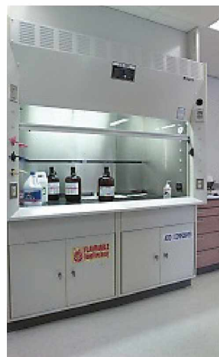
Figure 8. Laboratory chemical hood (note that the work area is inside the hood)
