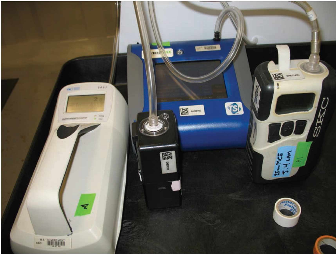
Figure 18. Area sampling for airborne nanomaterials
