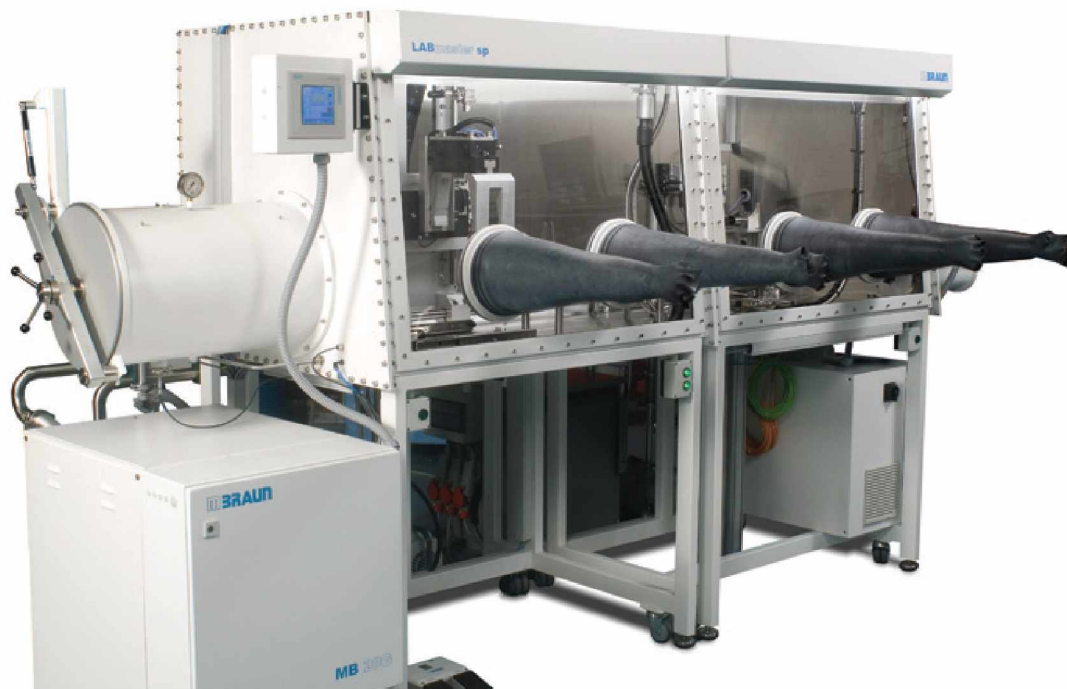
Figure 13. Glove box enclosure (shown here under positive pressure for use with inert atmospheres, rather than for enhanced containment of particles and gases)(MBRAUN; used with permission).
