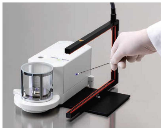
Figure 17. Example of a U-Frame antistatic device being used with a microbalance (photo courtesy of METTLER TOLEDO).
