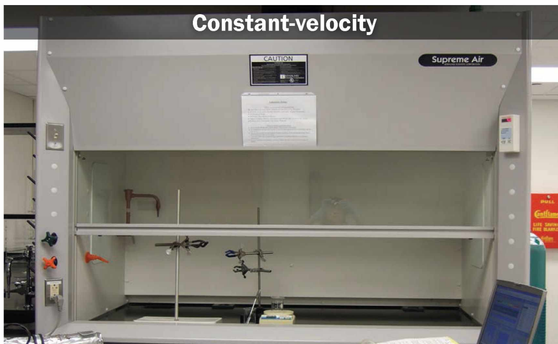
Figure 12. Laboratory constant-velocity hood (note the flow monitor on the sash column)
