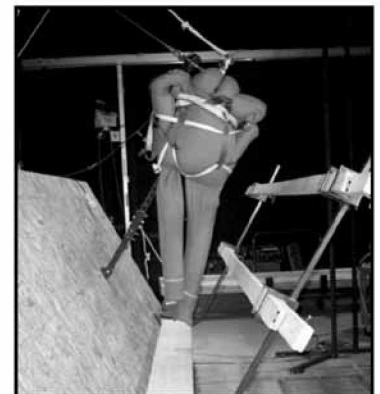
Figure 1. Test set-up with manikin ready to fall against top rail.
