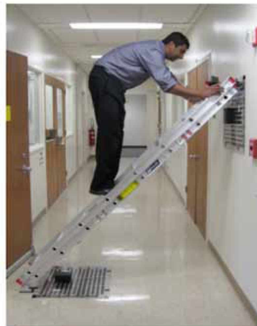
Figure 2. Ladder (at an otherwise unsafe angle) with electroadhesive pads active
