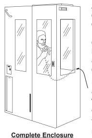
A fully enclosed booth or tent is the preferred type of local exhaust device. These devices physically separate the patient from others during sputum induction. Air from booths and tents is usually HEPA-filtered and discharged back into the room, but can also be exhausted outdoors. Some booths and tents can be easily assembled, dismantled, folded, and stored. Others are more difficult to assemble and disassemble, requiring greater installation time and effort.
