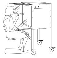
Patients must be instructed to sit as far as possible inside the hood opening when coughing. The hood should maintain an air velocity of at least 200 feet per minute (FPM) at the patient's breathing zone to capture droplet nuclei. Air currents from open windows and doors, or people moving about the room, can adversely impact the effectiveness of these devices. Partial enclosures are commonly mounted on carts that can be moved to any room for sputum induction procedures.
