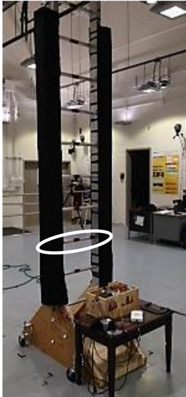
Figure 1: Instrumented ladder with electronically-controlled breakaway rung. The ellipse encircles the breakaway rung.
