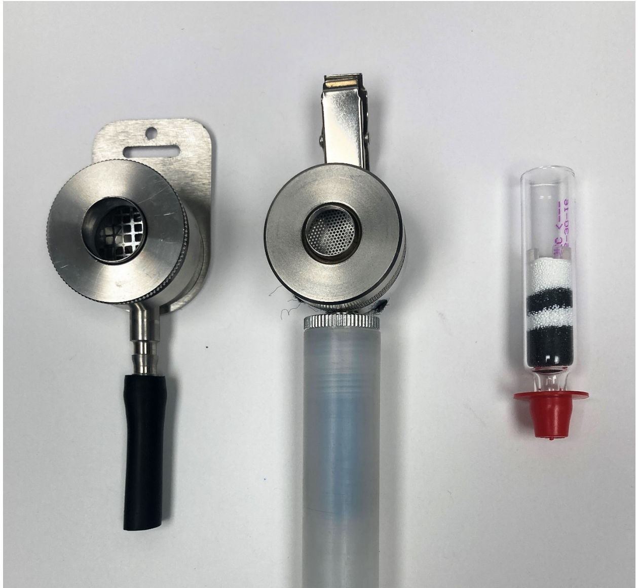
Figure S2: The stainless-steel IOM sampler, IVF Pro Sampler, and OVS, respectively.
