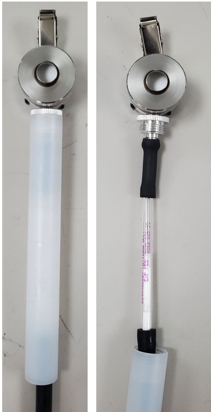
Figure S3: SKC IFV Pro with protective sheathe, and sorbent tube assembly.
