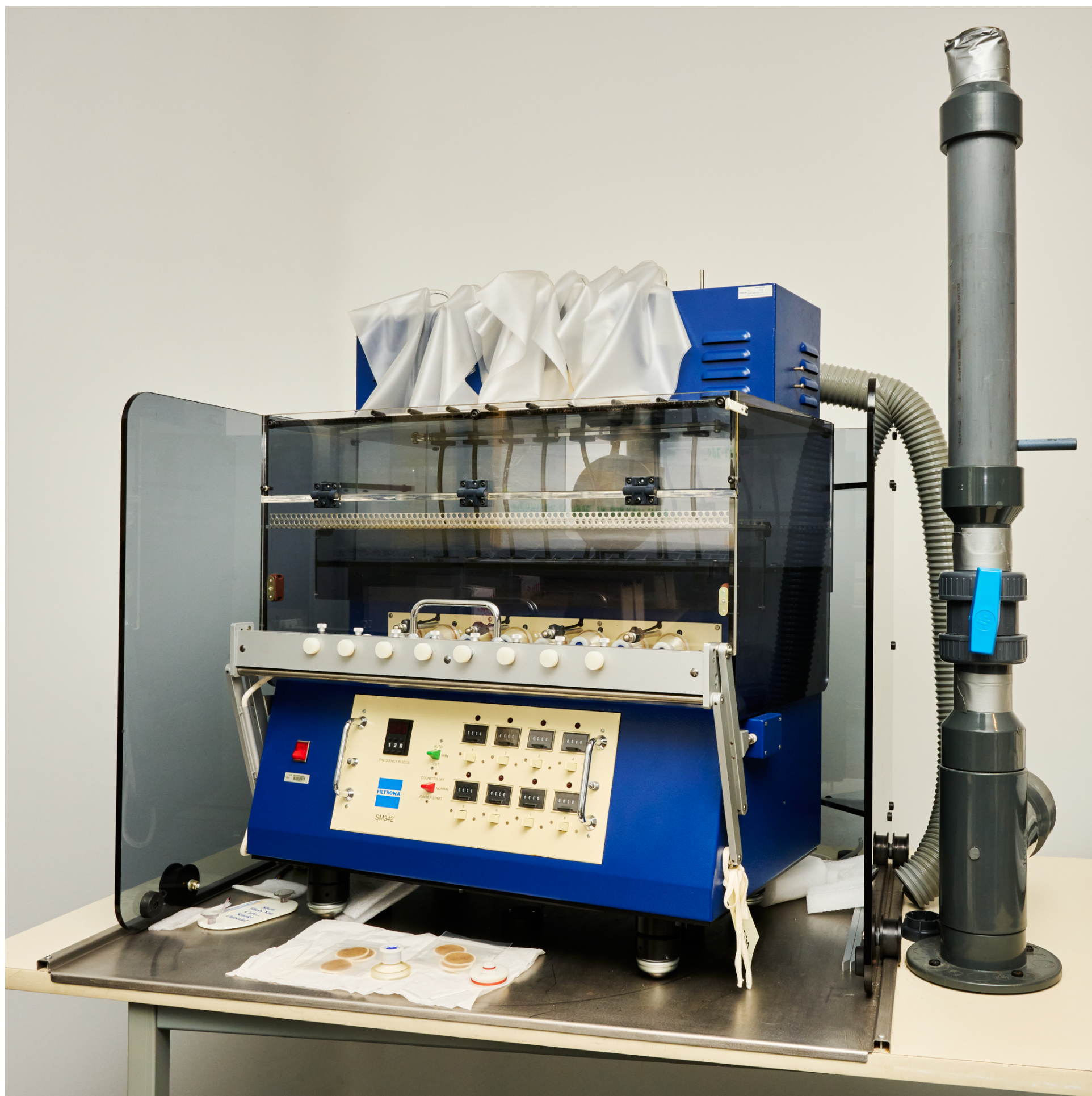
Harmonized 8 Channel Smoking Machine (1994) that was used by the CDC Tobacco Laboratory till the early 2000s.
