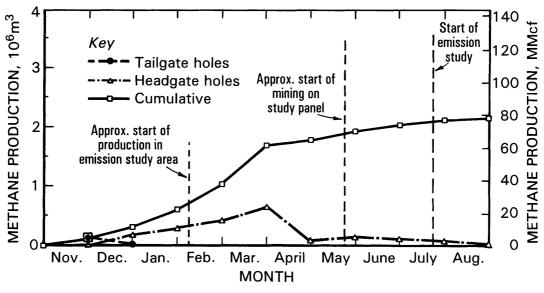
Figure 28.—Horizontal methane drainage borehole production, VP-1 Mine study panel.
