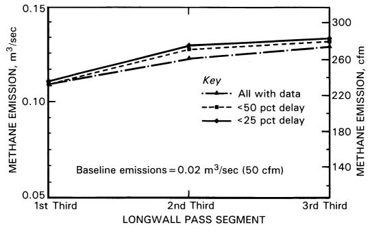
Figure 5.—Average methane emissions by pass segment, VP-1 Mine.
