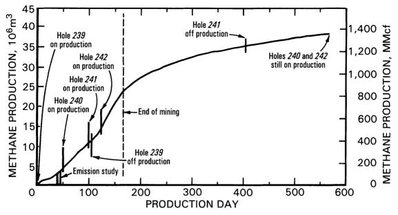
Figure 32.-Cumulative gob gas venthole methane production, VP-1 Mine safety panel.
