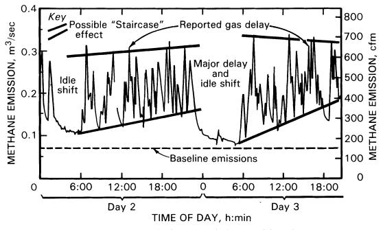
Figure 17.—Longwall face methane emission intervals exhibiting a possible "staircase" effect, days 2 and 3, VP-3 Mine.
