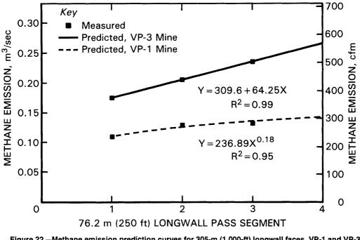
Figure 22.—Methane emission prediction curves for 305-m (1,000-ft) longwall faces, VP-1 and VP-3 Mines.
