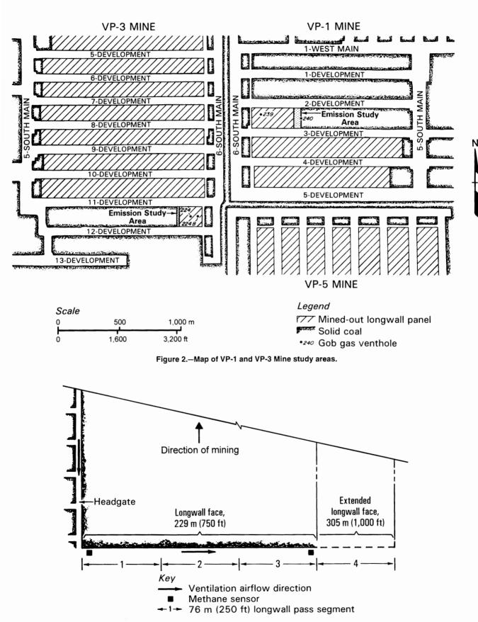
Figure 3.—Plan view of longwall face divided into equal-length segments for analysis and prediction of methane emission trends.
