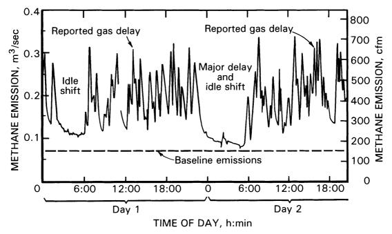
Figure 13.-Longwall face emissions for days 2 and 3, VP-3 Mine.
