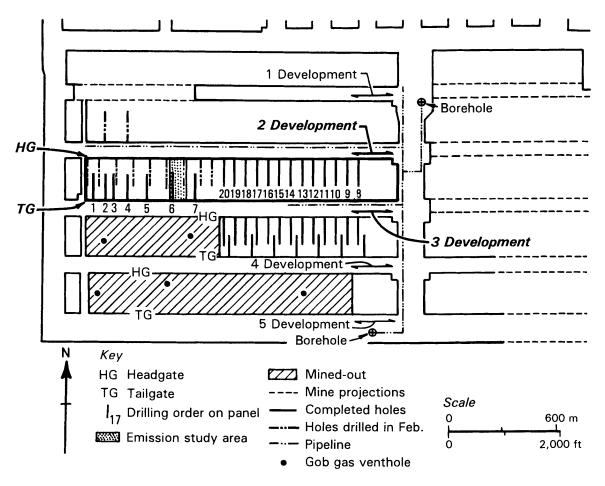
Figure 27.-Location of horizontal methane drainage boreholes, VP-1 Mine study panel.
