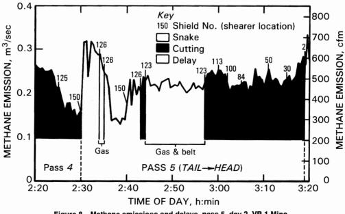
Figure 8.-Methane emissions and delays, pass 5, day 2, VP-1 Mine.
