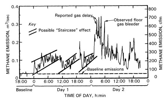
Figure 10.-Longwall face methane emission intervals exhibiting a possible "staircase" effect, day 1, VP-1 Mine.
