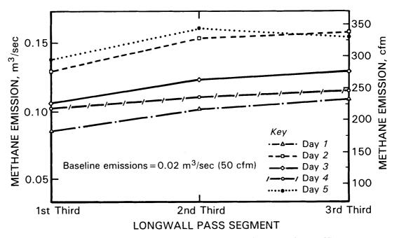
Figure 6.—Average daily methane emissions, all passes with data basis, VP-1 Mine.
