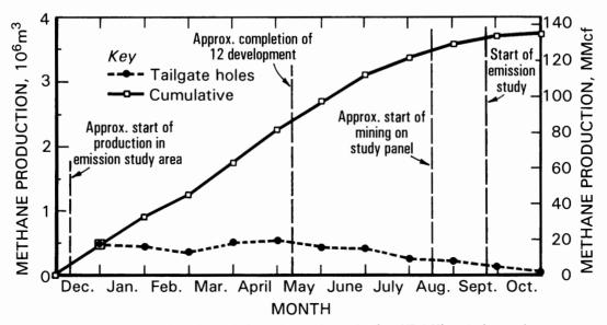
Figure 30.—Horizontal methane drainage borehole production, VP-3 Mine study panel.
