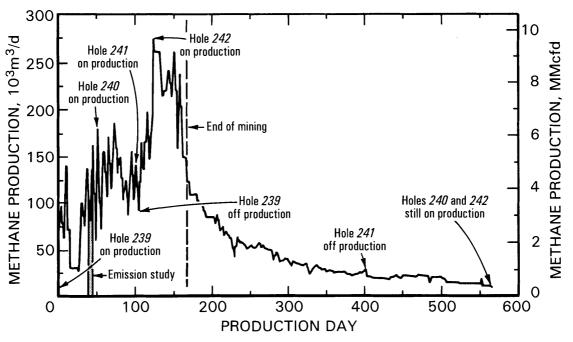
Figure 31.—Daily total gob gas venthole methane productions, VP-1 Mine study panel.
