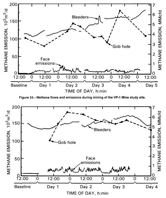
Figure 25.—Methane flows and emissions during mining of the VP-3 Mine study site.
