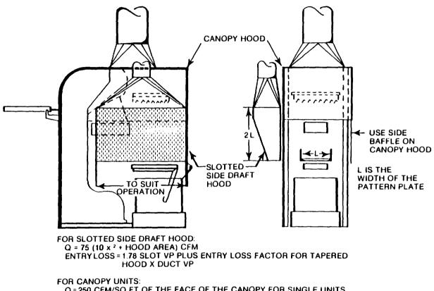
Q = 250 CFM/SQ FT OF THE FACE OF THE CANOPY FOR SINGLE UNITS = 150 CFM/SQ FT OF THE FACE OF THE CANOPY FOR DOUBLE UNITS ENTRY LOSS = ENTRY LOSS FACTOR FOR TAPERED HOOD X DUCT VP
