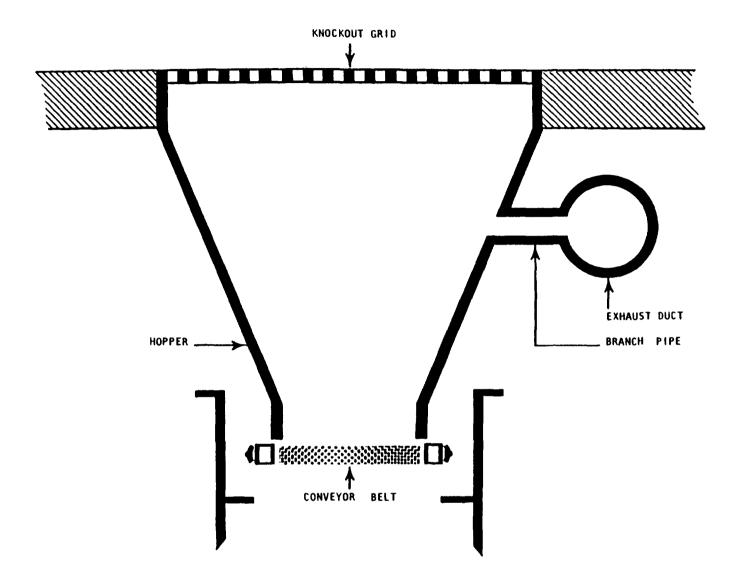
FIGURE IV-3. Local exhaust ventilation below knockout grid
