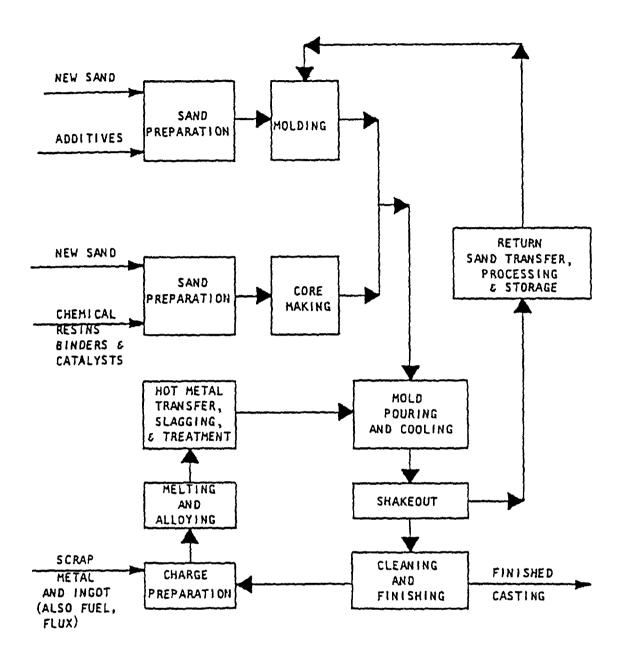
FIGURE 11-1. Schematic diagram of overall foundry process
