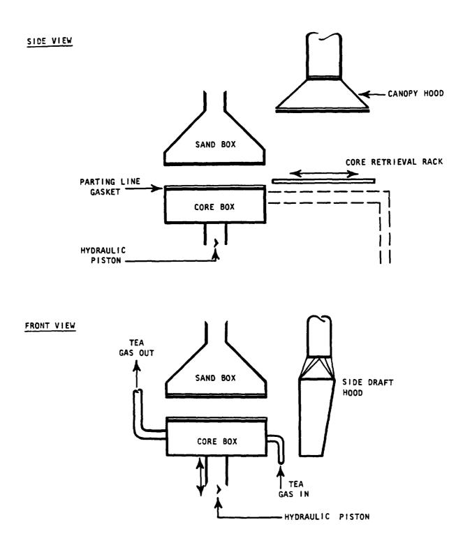
FIGURE IV-12. Cold-box coremaking exhaust
