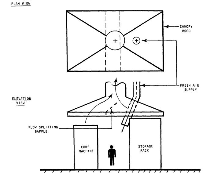
FIGURE IV-11. Canopy hood and fresh air supply for furan hot-box core machine
