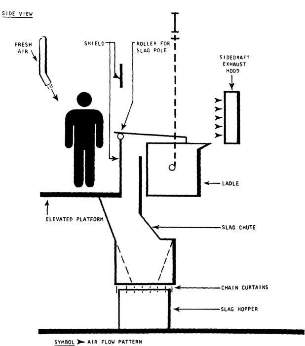
FIGURE IV-13. Slagging station
