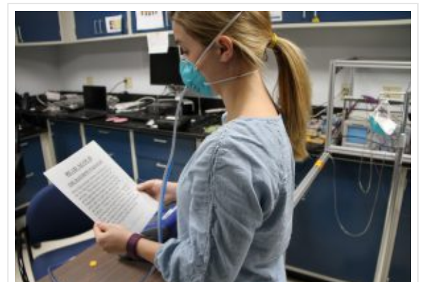
An individual reading the 'Rainbow Passage' during a respirator fit test. Photo from NIOSH
