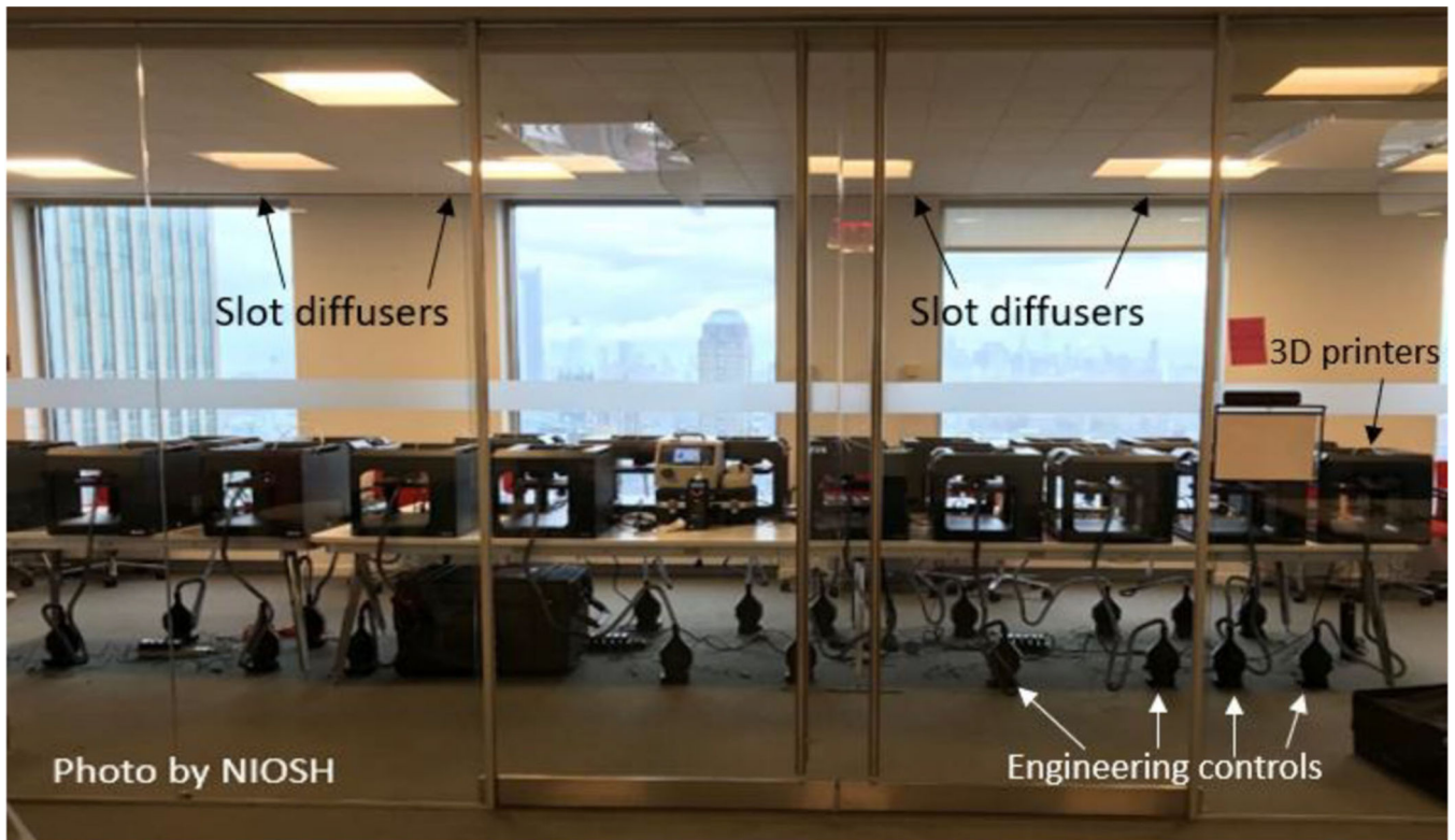
Fig. 2. Twenty MakerBot Replicator+3D printers with LEV engineering controls in a simulated makerspace (aka conference room). Photo by NIOSH
