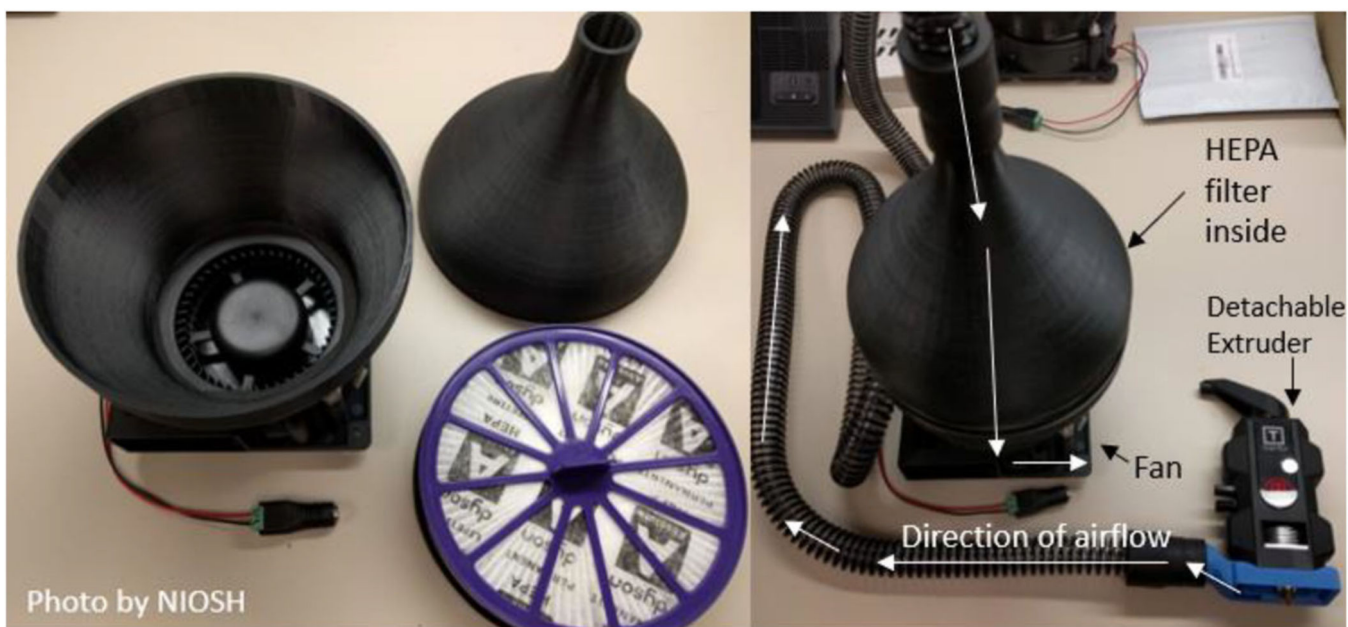
Fig. 4. Low-cost air cleaner assembly connected to a modified smart extruder cover. The HEPA filter is 14 cm (5.5 in) in diameter and 2.5 cm (1 in) in thickness
