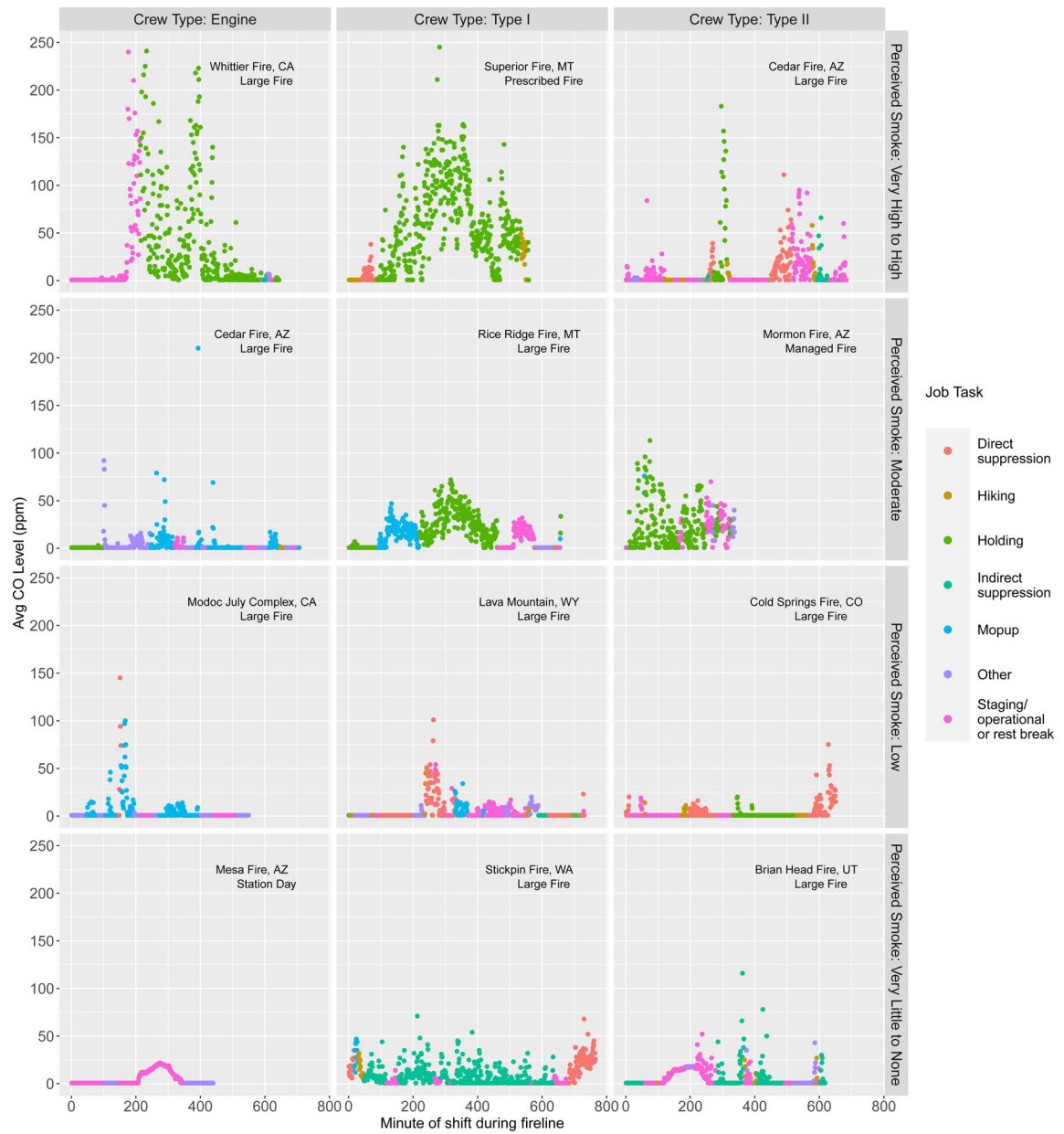
Figure 1. CO exposure by job task, crew type, and perceived smoke exposure for selected WFFs during a single shift. CO concentrations exceeding 250 ppm are not shown in the plots but occurred for 16 minutes during the Whittier fire, and for 1 minute for during the Superior, Cedar (Type II), and Modoc July Complex fires.
