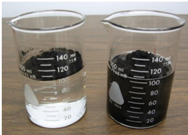
Figure 4.16. Hydrophobic coal floating on water and sinking with the addition of a wetting agent (left) and a bar chart representing changes in airborne dust capture with wetting agents (right).
