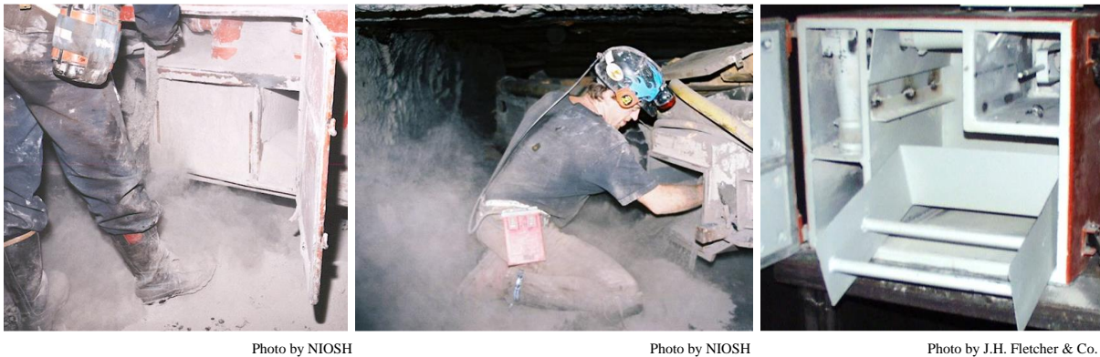
Figure 4.21. Dust dropping out of dust box (left), operator cleaning dust box by hand (center), and insert used to assist in cleaning of dust box (right).
