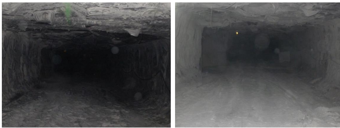
Figure 6.5. Return entry after a cut without (left) and with flooded bed scrubber operating (right) illustrating difference in float coal dust deposition.
