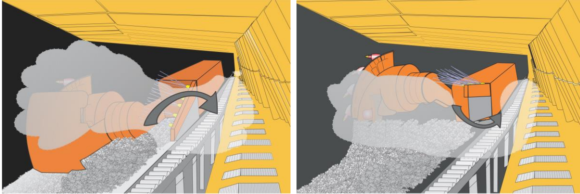
Figure 3.26. Illustrations of splitter arm in a lowered position during the head-to-tail pass (left) and in a raised position during the tail-to-head pass (right). These positions may allow dust to migrate into the walkway on higher-seam longwalls.
