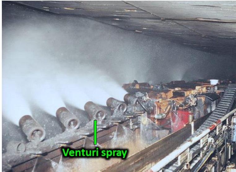
Figure 3.22. Venturi sprays mounted on headgate splitter arm.
