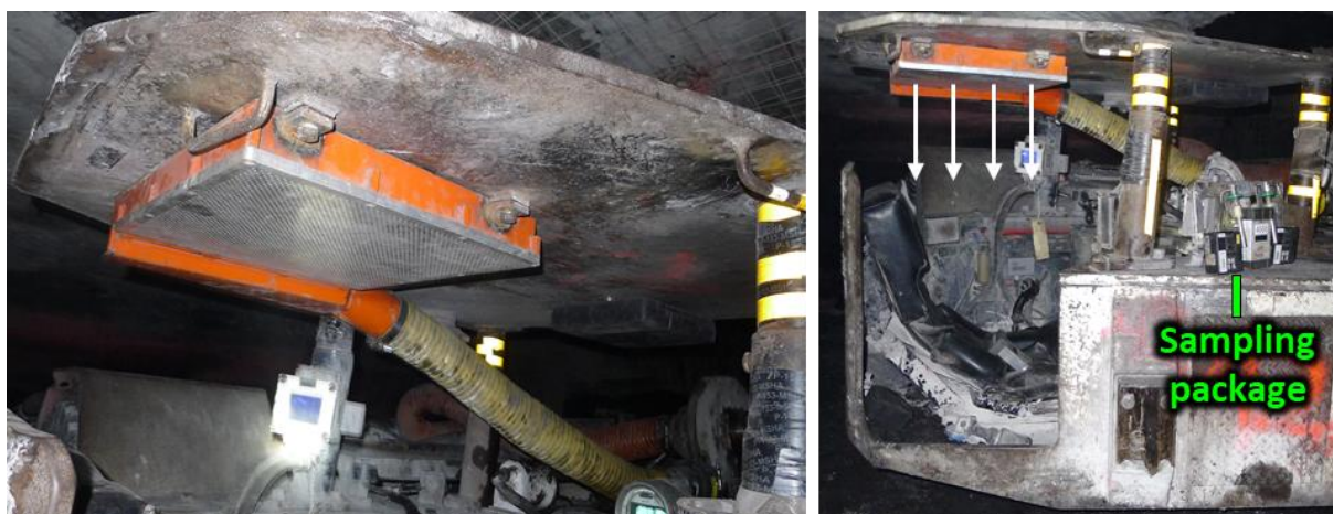
Figure 4.27. Canopy air curtain installed on underside of ram car canopy (left) and showing how filtered air is blown down over operator's position, along with a dust sampling package located outside of cab (right). White arrows indicate airflow.
