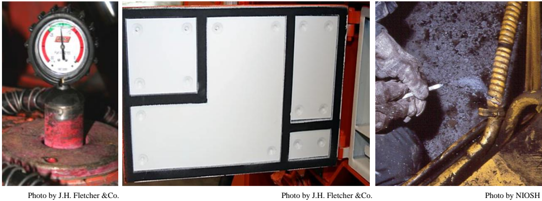
Figure 4.20. Methods to ensure dust collector performance. A gauge is placed in the drill chuck to measure vacuum at the drill head (left), gaskets (in black) on the door of dust collector box are checked (center), and smoke tubes can be used to check for leaks in the system (right).
