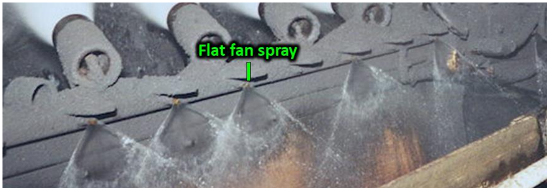
Figure 3.23. Flat fan sprays mounted on walkway side of belting on the headgate splitter arm.
