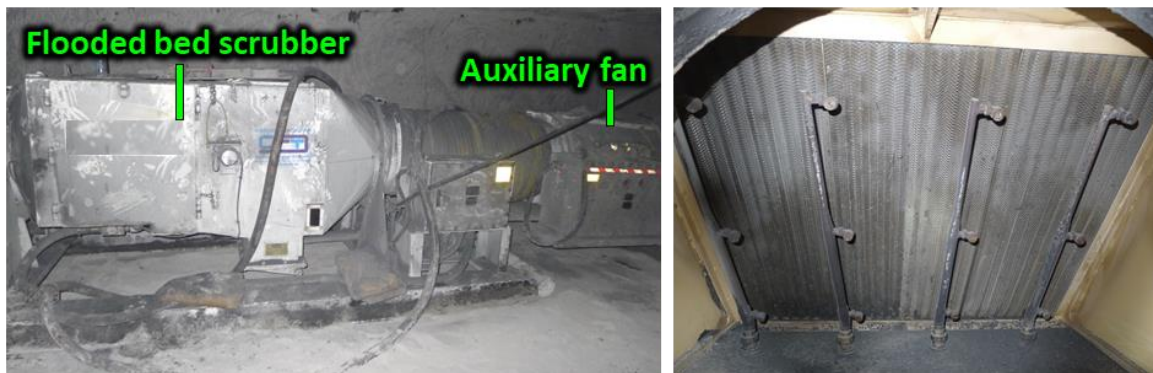
Figure 6.4. Flooded bed scrubber unit (left) and 12 water sprays used to wet filter panel (right).
