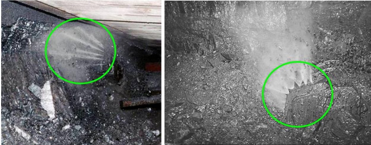
Figure 3.28. Crescent sprays mounted on shearer ranging arms.
