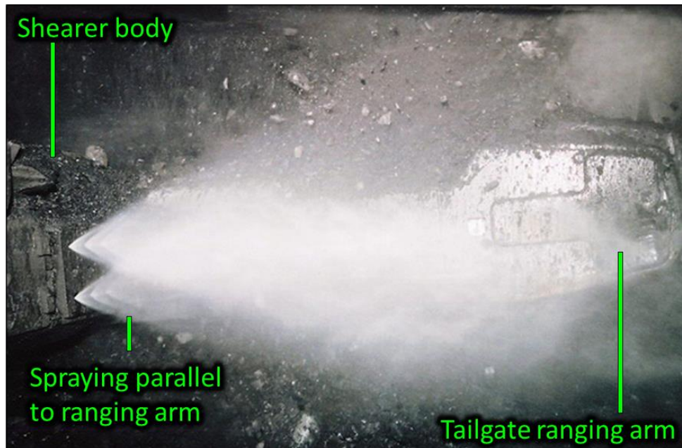
Figure 3.25. Sprays mounted on tailgate end of shearer body and directed parallel to ranging arm.
