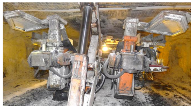
Figure 4.24. Canopy air curtains installed on roof bolters at two underground coal mines.
