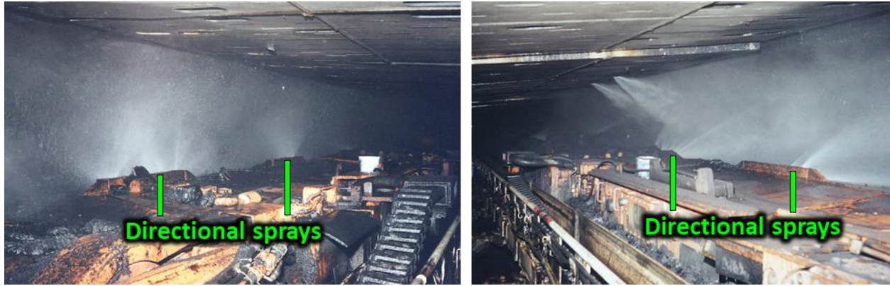
Figure 3.24. Directional spray manifolds mounted on face side of shearer body as viewed from the headgate (left) and tailgate (right) sides of the shearer.
