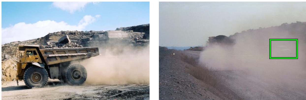
Figure 5.12. Examples of haul road dust generated by haul trucks. In the photo on the right, the green box outlines a pickup truck and illustrates the loss of visibility from dust obstruction.
