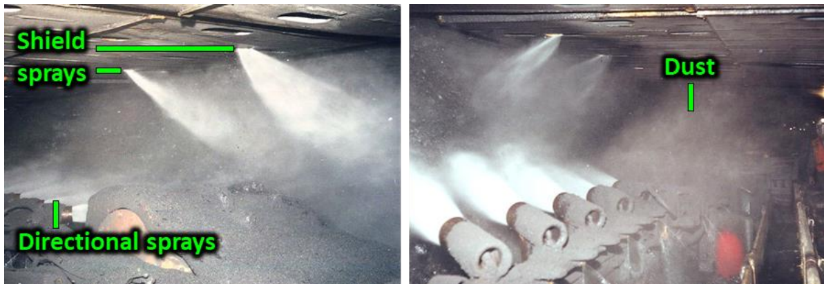
Figure 3.31. Shield sprays located on the underside of the canopy interacting with directional sprays on the shearer (left), allowing dust to move toward the walkway (right).
