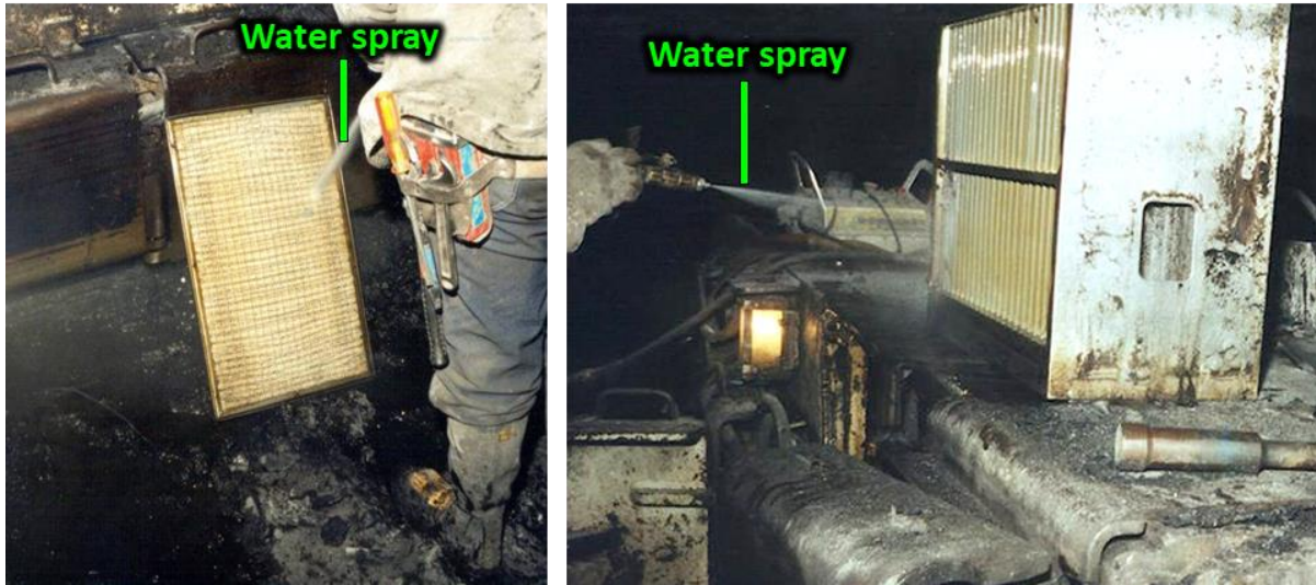
Figure 4.15. Cleaning scrubber filter panel (left) and mist eliminator (right) with a water spray.
