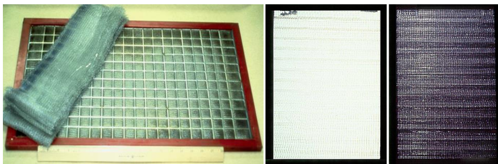
Figure 4.13. Forty-layer flat filter panel with mesh material shown (left). Ten-layer (center) and 30-layer (right) pleated panels with backlighting to show relative difference in filter density.
