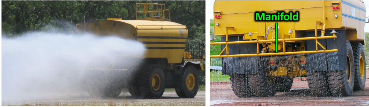
Figure 5.14. Water trucks wetting haul roads with rear-mounted water sprays (left) and a water distribution manifold (right).
