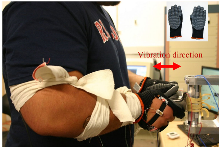
(a) A pictorial view of the simulation of a worker holding a workpiece (golf club head) and pushing against a simulated grinding interface
