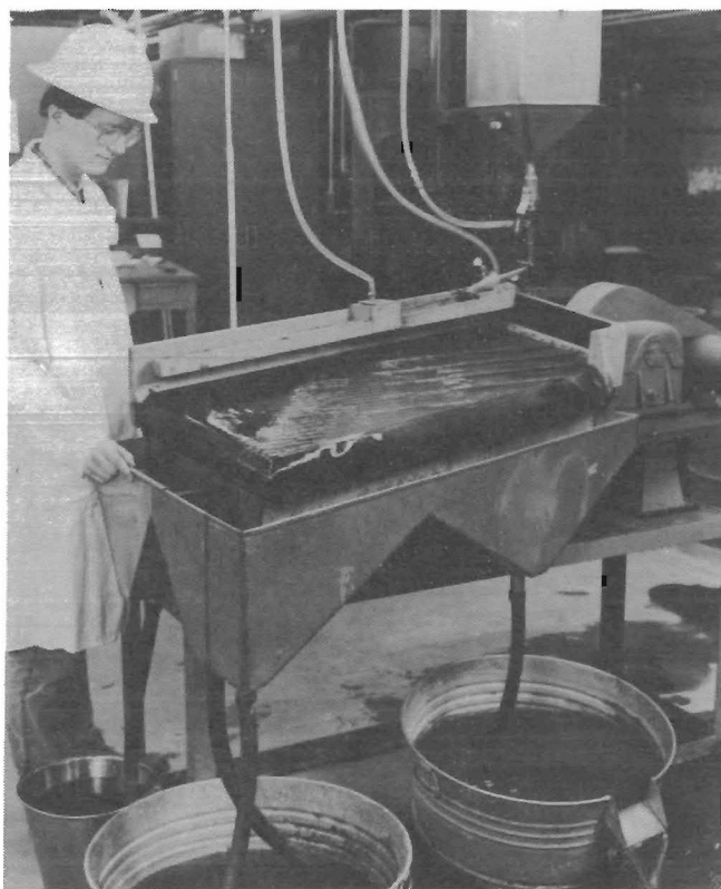
Figure 3.—Deister table used to concentrate scheelite.
