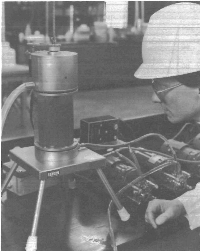
Figure 6.—High-rate thickener sizing test unit.
