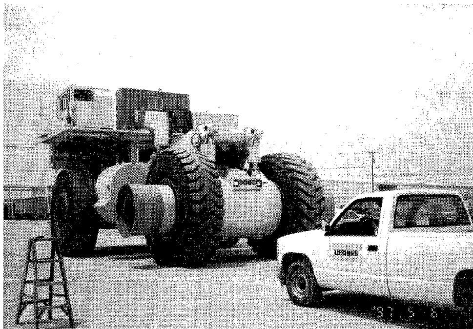
Doppler radar backup alarm being tested on 240-ton class mining truck
