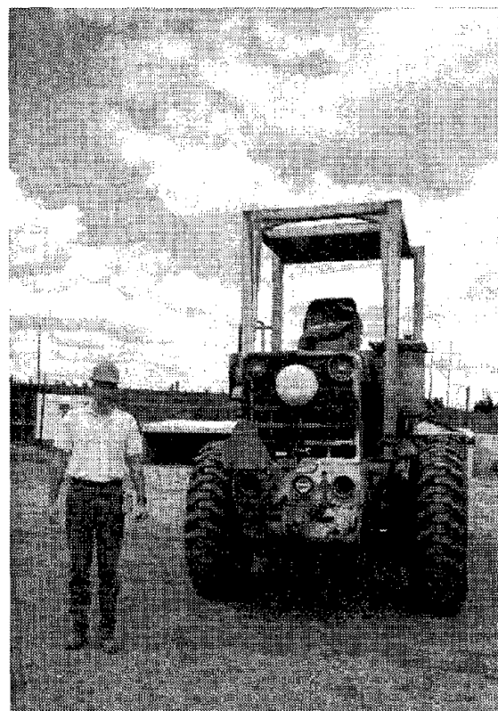
The collision avoidance sensor is mounted on a front-end loader while the tag is worn on the pedestrian's belt.
