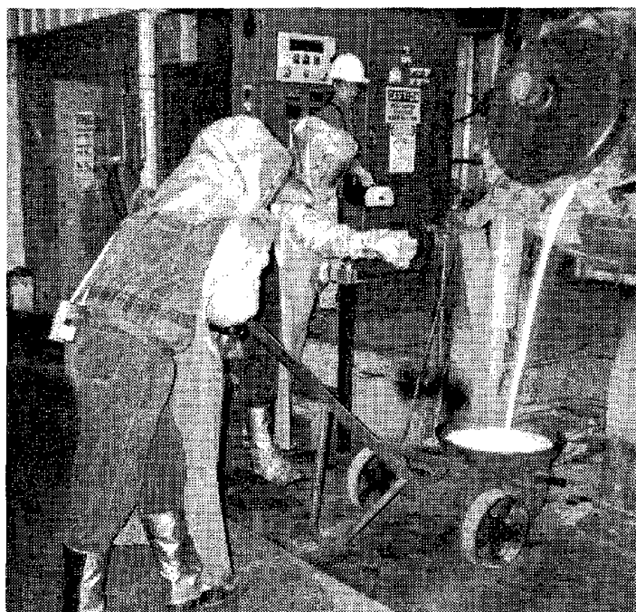
Project personnel conducting spot checks for mercury vapor during a pour of molten slag.
