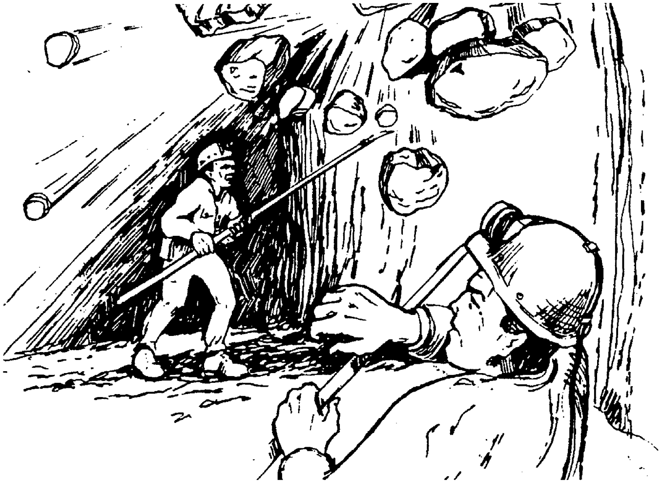
The obvious hazards of scaling loose rock
