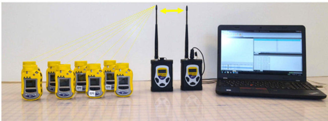
Figure 2. Eight PID gas sensors wirelessly connected to long range modems wired to a laptop with data acquisition software.
