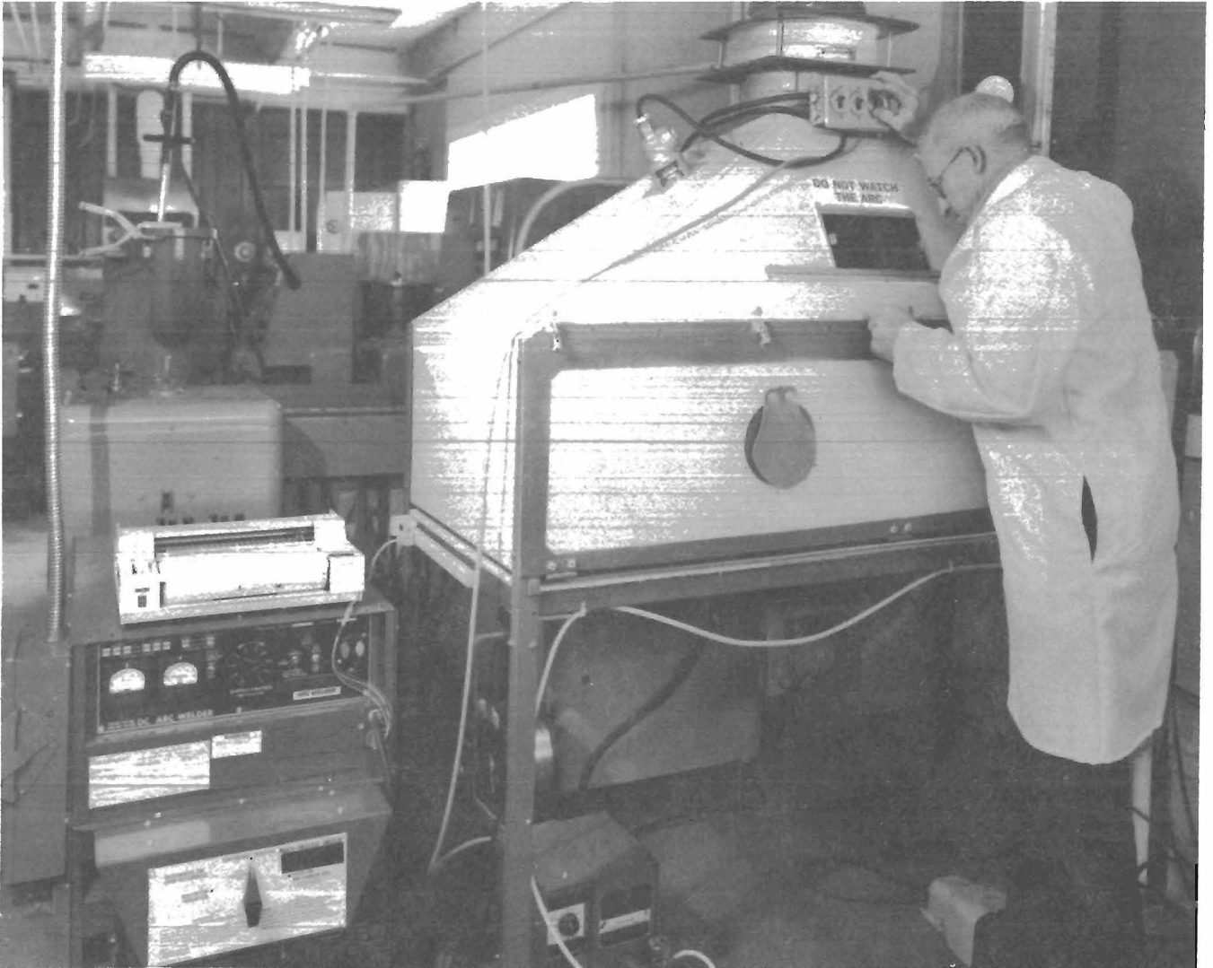
FIGURE 1. - Operator preparing to strike an arc using an automatic wire feed. The welding operation inside the chamber is viewed through a filtered glass plate positioned across the view port. Fumes generated are swept up to a filter housed just above the operator's right hand by a suction blower (not shown). The power supply, strip chart recorder for voltage and current measurement, and wire feed unit are seen at left and below the chamber.
