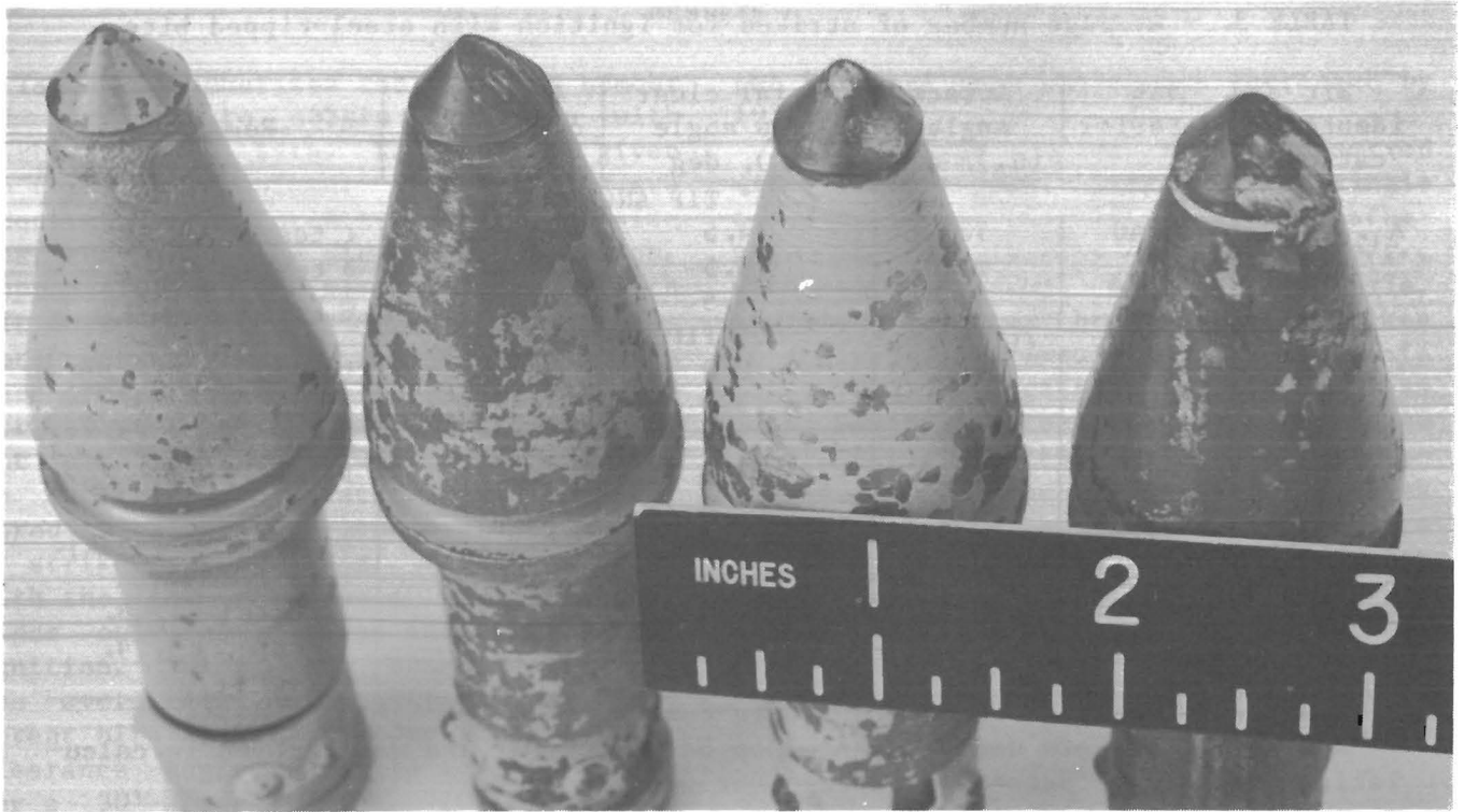
FIGURE 4.—New (left) and used tungsten-carbide-tipped (middle left and right) and steel-tipped (right) bits after ignition. (Bit tip angle, 80°; bit attack angle, middle left, 50°; middle right, 67°; right, 54°.)
