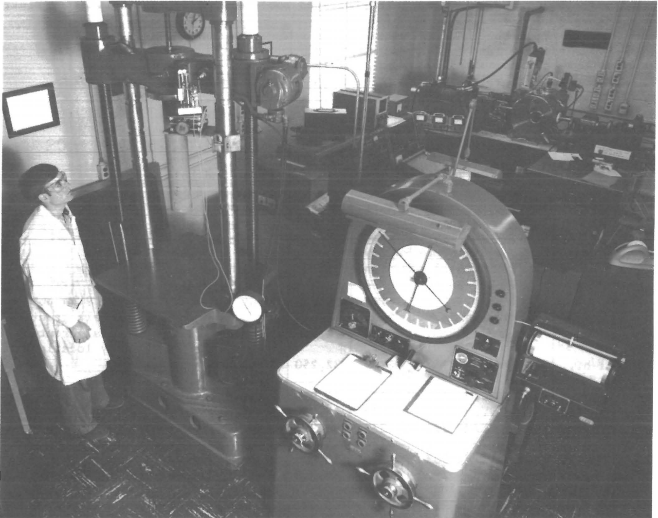
FIGURE 9. - Pull testing a 2-ft simulated roof-bolt system on universal hydraulic test machine.
