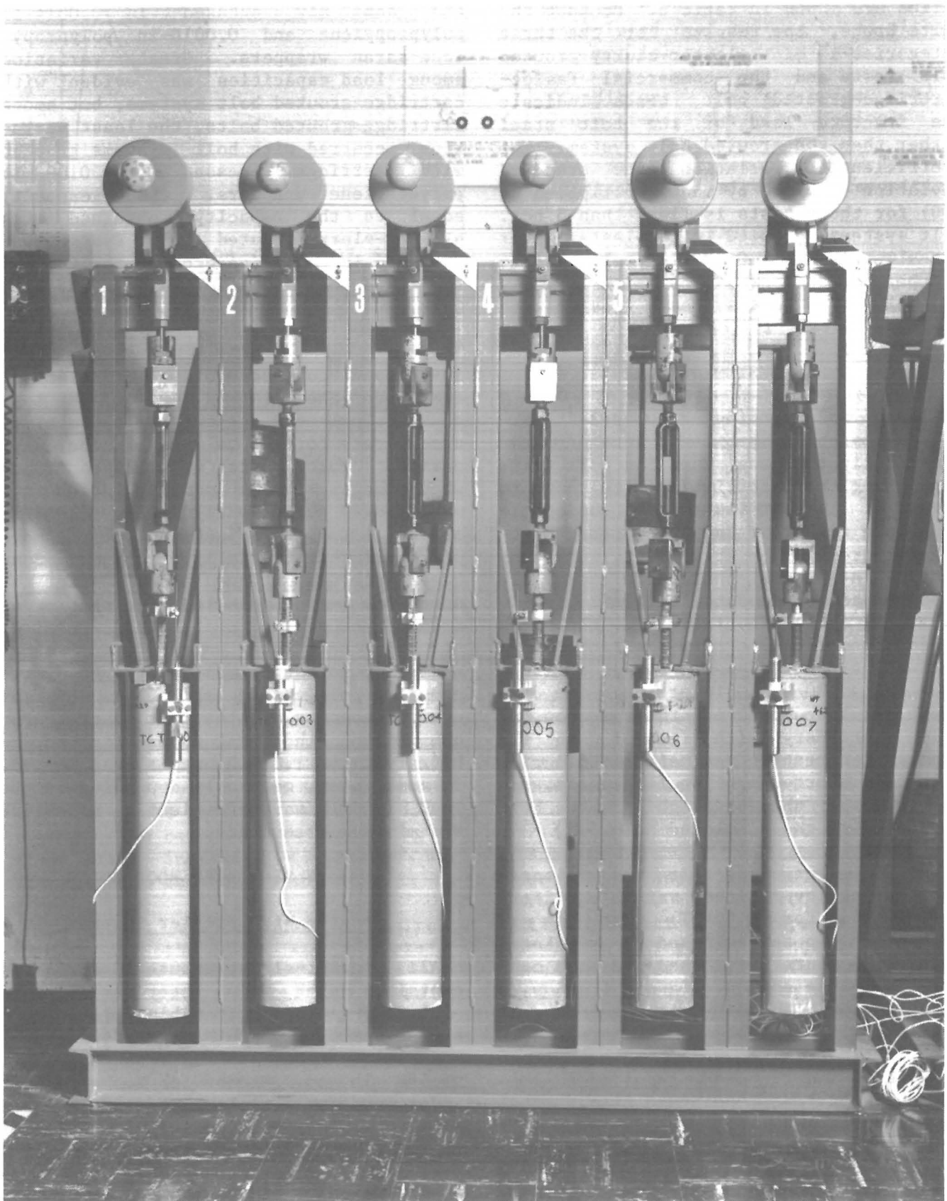
FIGURE 19. - Creep test frame loaded with six 2-ft simulated roof-bolt specimens.
