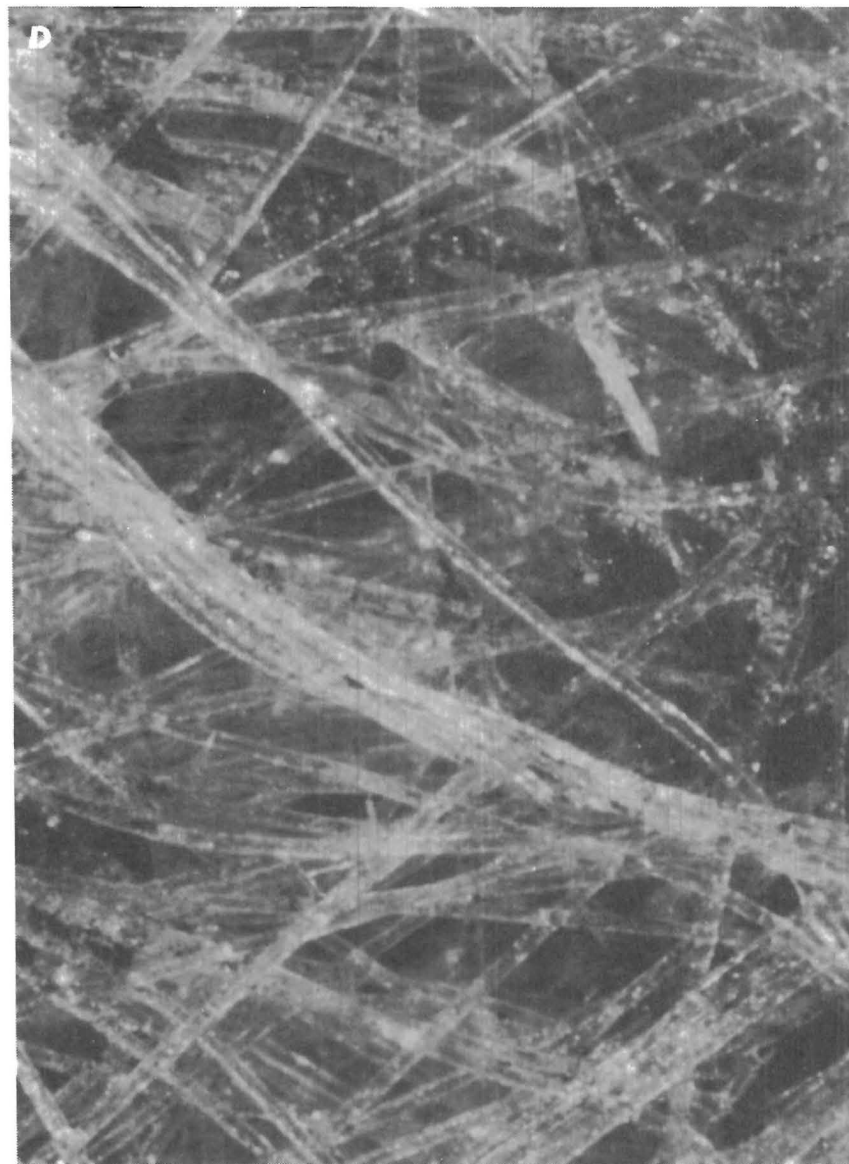
FIGURE 5. - Unused and used Mirafi 140S cloth samples (magnified)—Continued. C , Clogged area; D , waste trapped within fabric.
