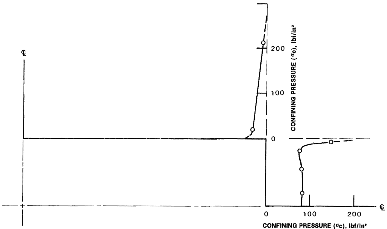
FIGURE 15. - Confining pressure distribution around coal mine entry.
