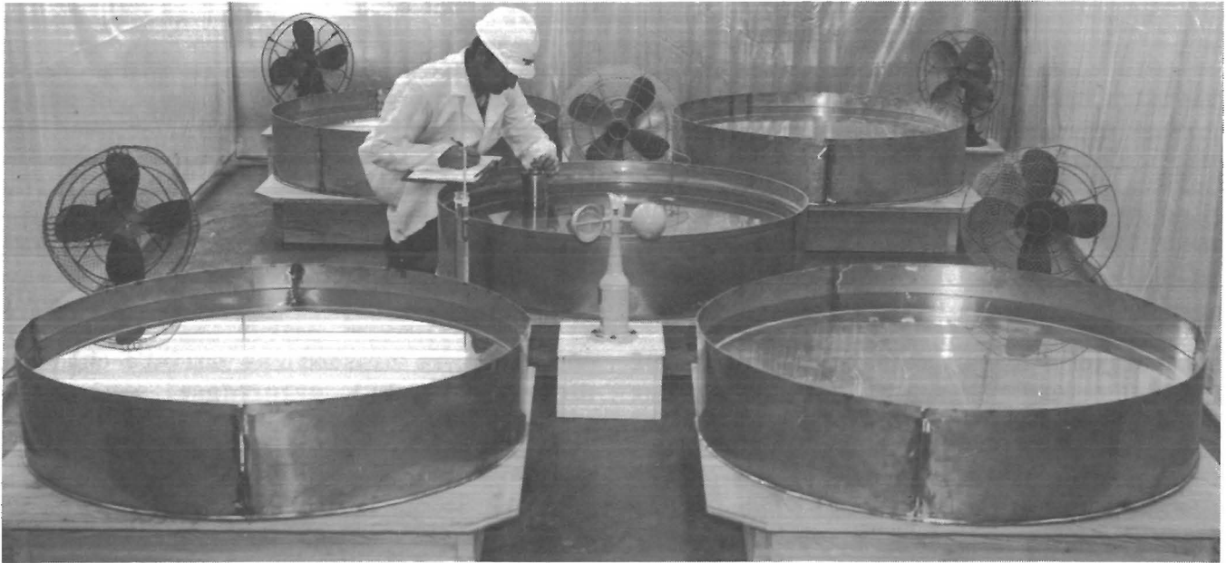
FIGURE 1. - Evaporation pans and monitoring equipment for potash brine evaporation studies.
