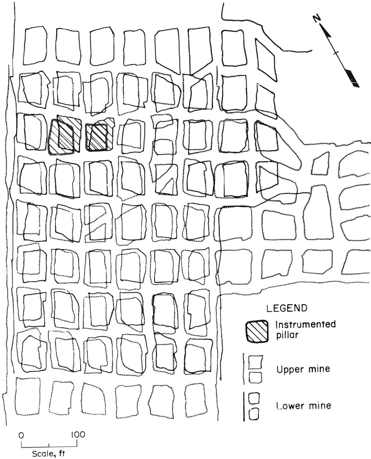
FIGURE 15.—Superpositioning of instrumented pillars.
