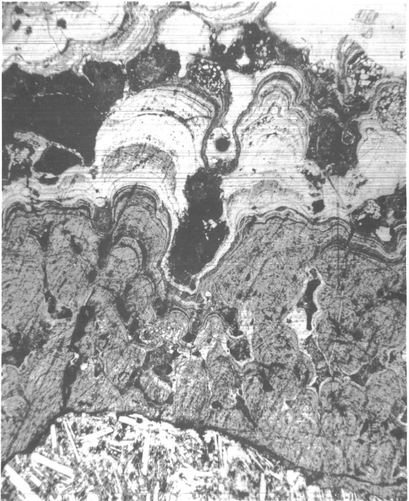
FIGURE A-7.—Sample O (X 32). Photomicrograph of polished section showing botryoidal manganese oxides at top, more iron-rich zones of manganese oxides in darker (tarnished appearance) middle zone, and trachytic sanidine substrate at bottom, with lath-shaped sanidine feldspar phenocrysts.
