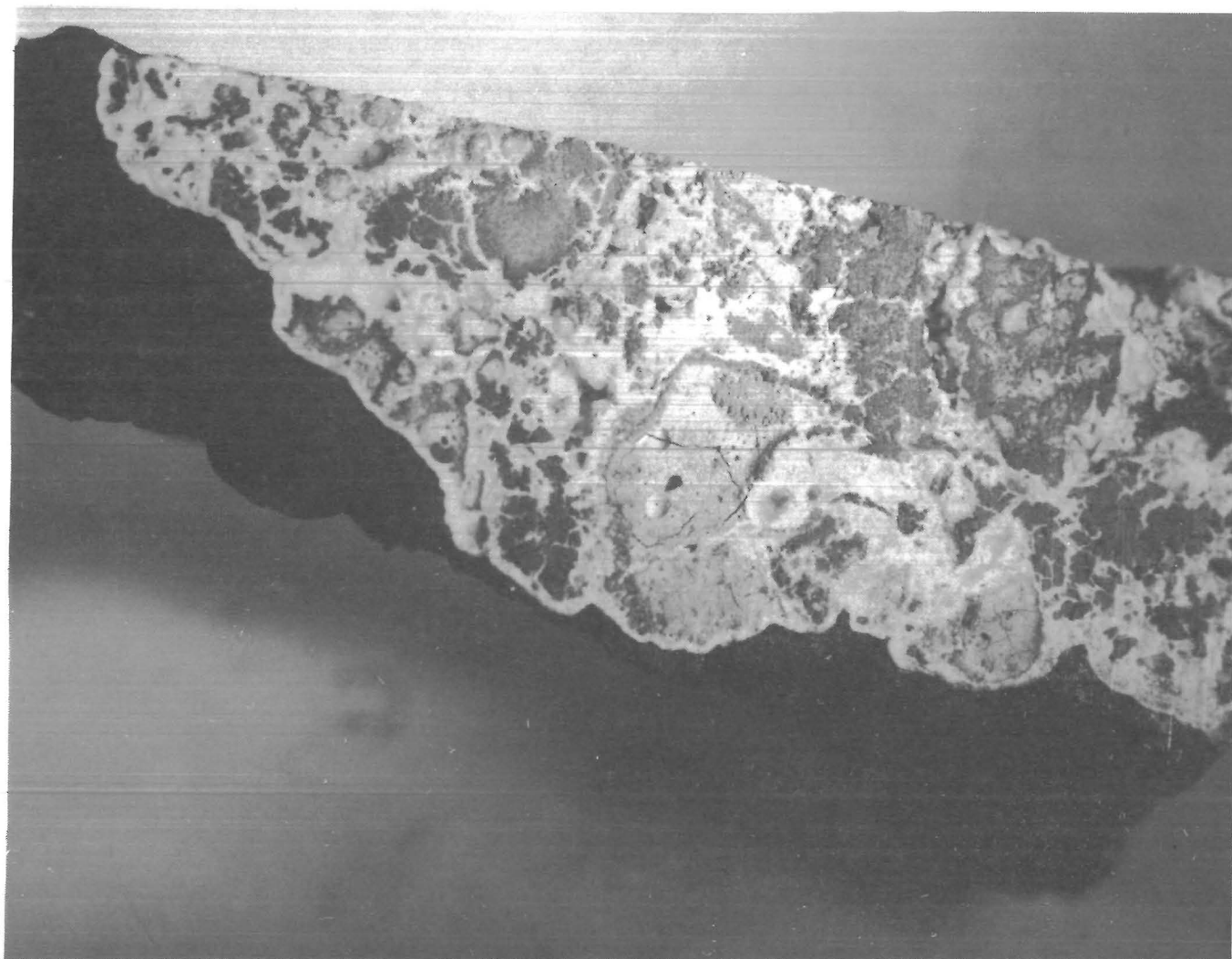
FIGURE A-6.—Sample D cross section (X 3). Substrate is altered basalt breccia, partially replaced by nontronite and encrusted with white to transparent layers of botryoidal phillipsite.
