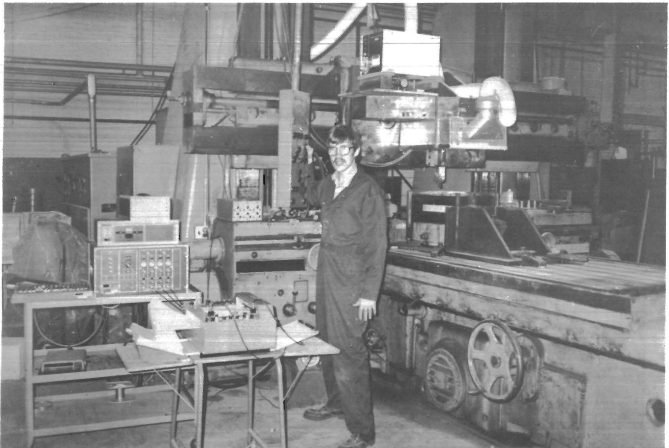
FIGURE 9.—Cutting test laboratory, milling machine in background and instrumentation in foreground.
