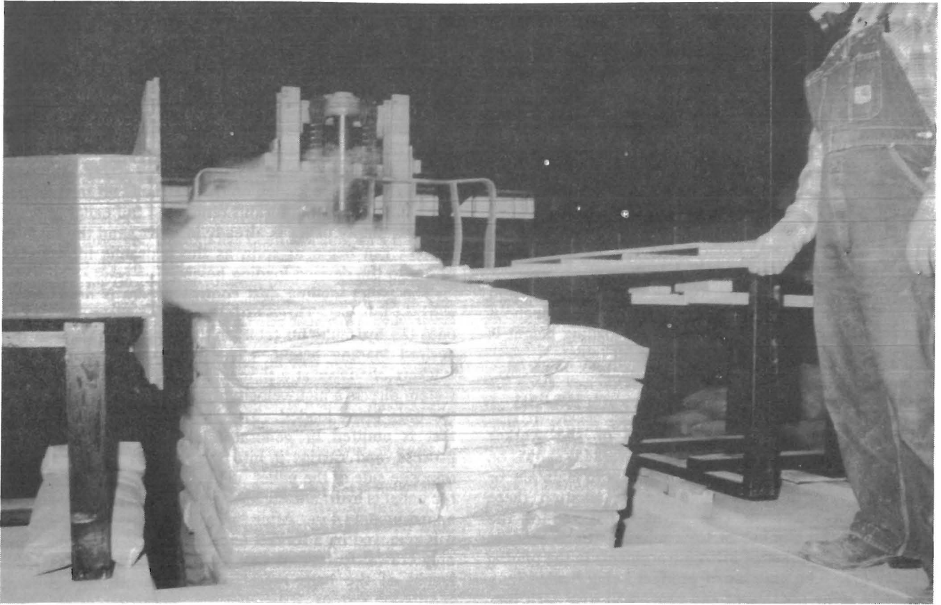
Figure 1.—Use of smoke to provide visual indication of system effectiveness.
