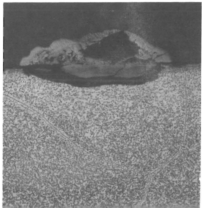
FIGURE 17. Cross section of localized oxidation (X 200) in Fe-12Cr-6Mo-1.75Ti alloy. Exposed 800 h at 700°C.
