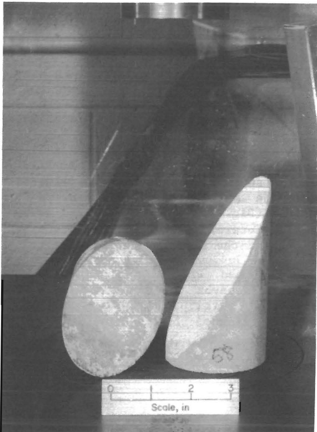
FIGURE 3.—Failure surface appearance when concrete exceeds strength of binder material.
