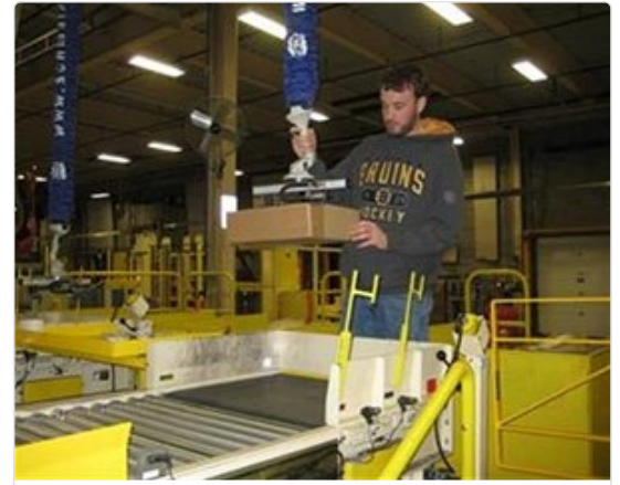
A materials-handling worker demonstrates using a vacuum-driven lift-assist device in an L.L.Bean warehouse.
