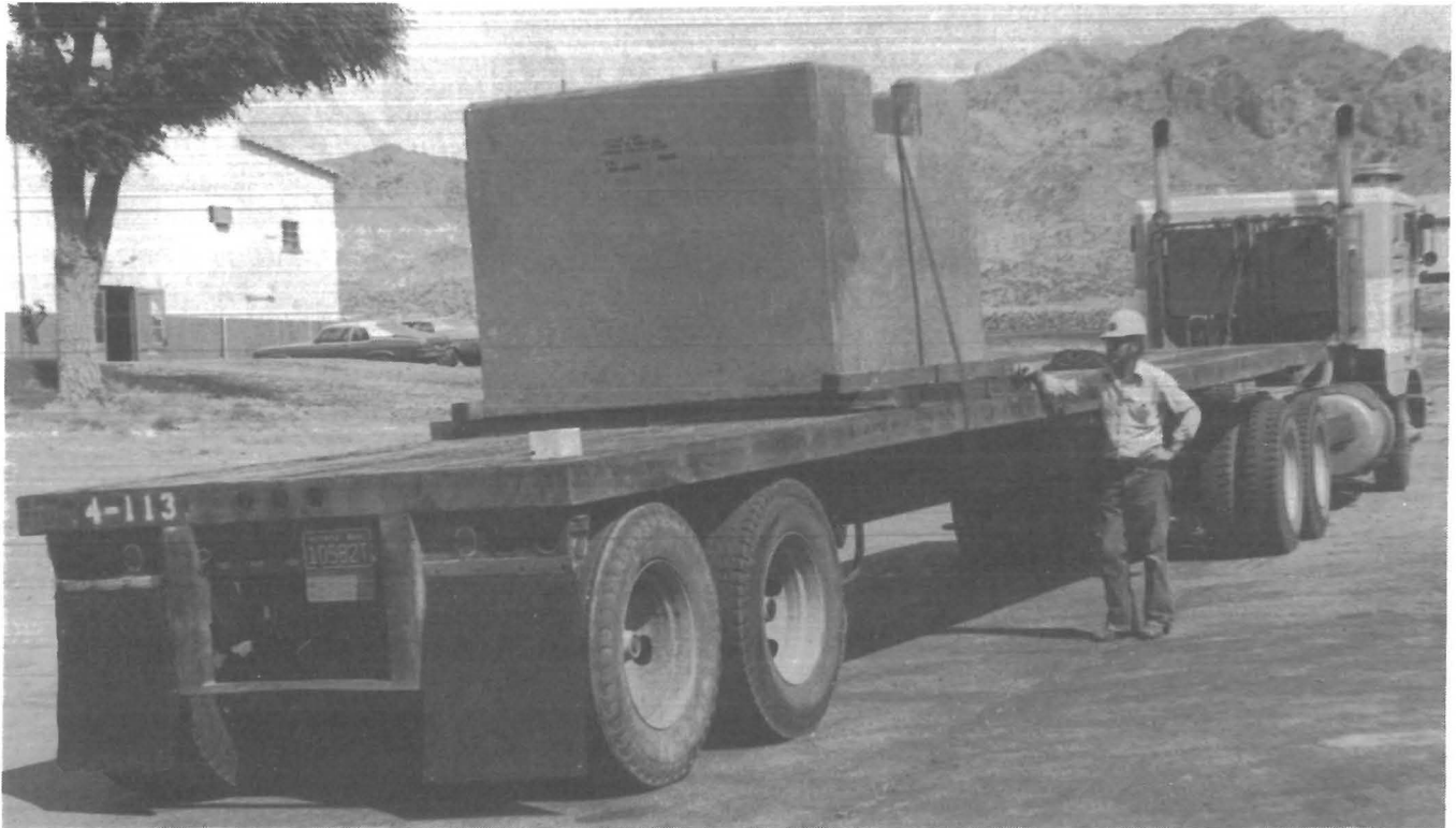
FIGURE 10. - Sulfur concrete sump unit for use in containing waste acidic solutions.
