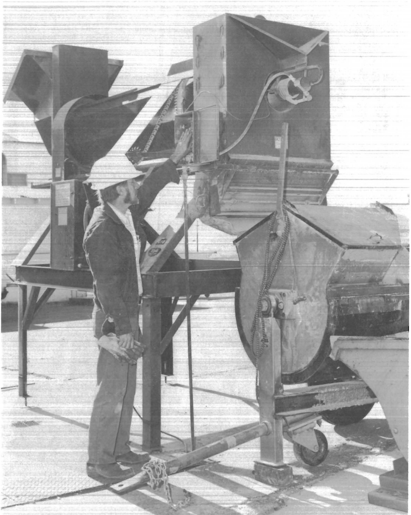
FIGURE 5. - Small-scale production unit for sulfur concrete.
