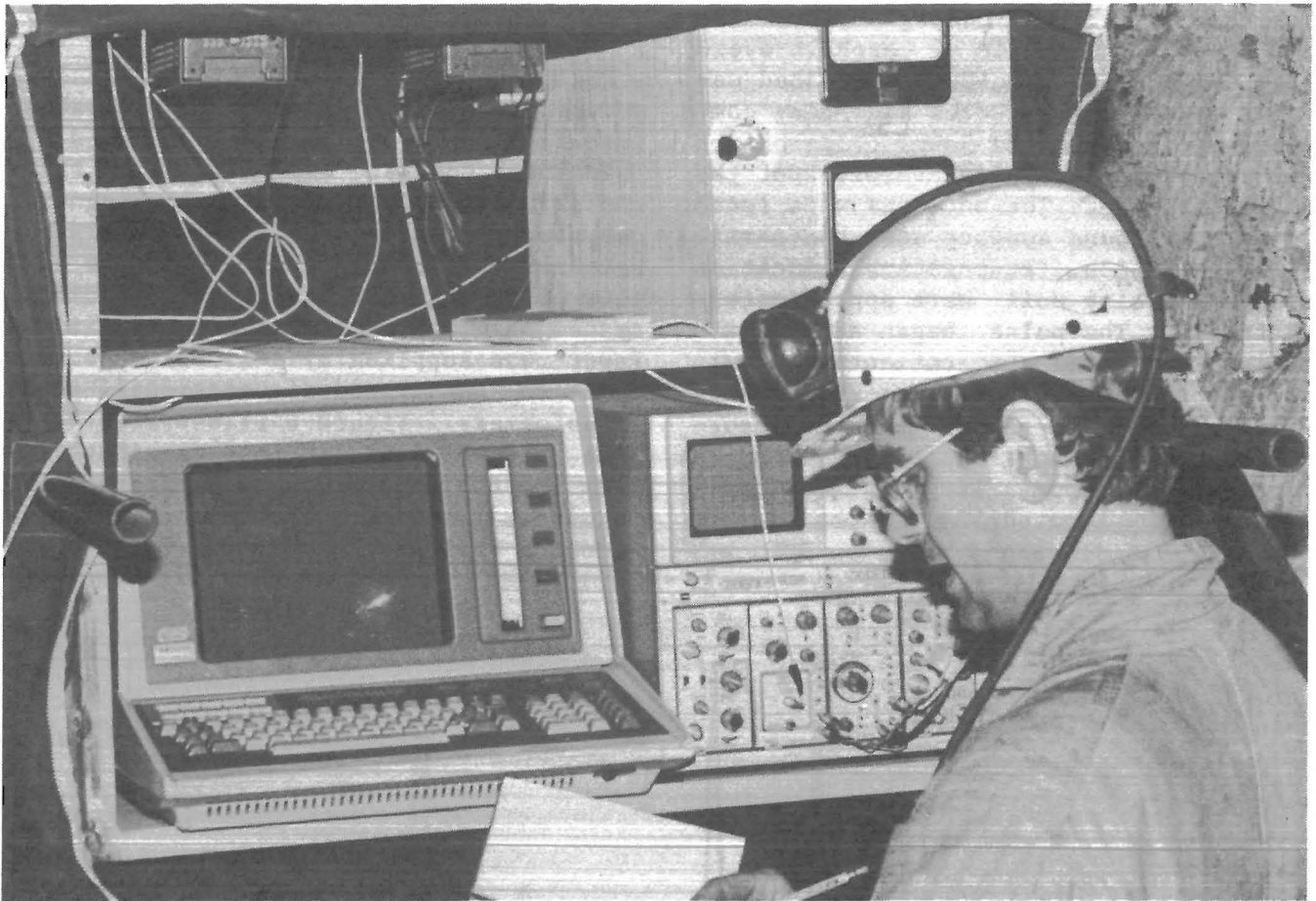
FIGURE 5. - GPR-operating control console.
